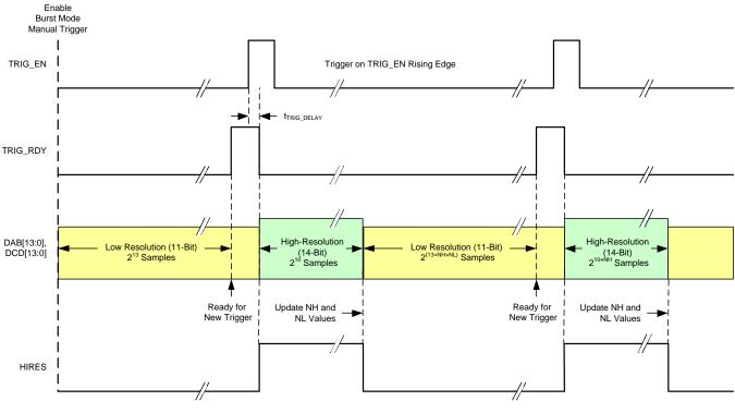
Figure 55. Timing For Manual-Trigger Mode
