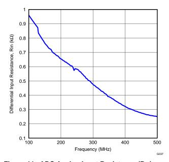
Figure 44. ADC Analog Input Resistance (R<sub>IN</sub>) vs Frequency
