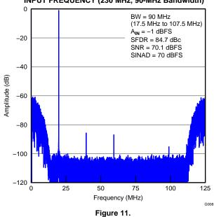
FFT IN 11-BIT MODE WITH SNRBoost<sup>3G+</sup> INPUT FREQUENCY (230 MHz, 90-MHz Bandwidth)
