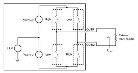
Figure 63. LVDS Buffer Equivalent Circuit
