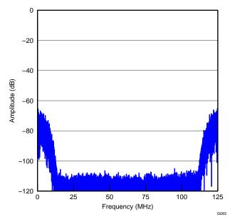
Figure 59. 90-MHz SNRBoost<sup>3G+</sup> Filter Bandwidth Centered on f<sub>S</sub> / 4
