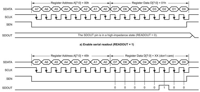
The SDOUT pin functions as a serial readout (READOUT = 1).
