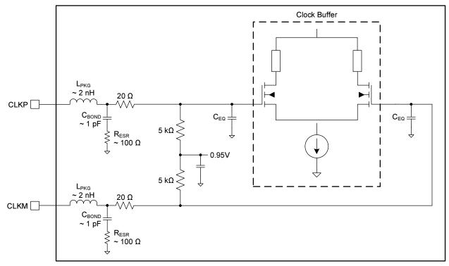
C<sub>EQ</sub> is 1 pF to 3 pF and is the equivalent input capacitance of the clock buffer.
