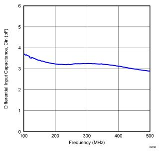
Figure 45. ADC Analog Input Capacitance (C<sub>IN</sub>) vs Frequency
