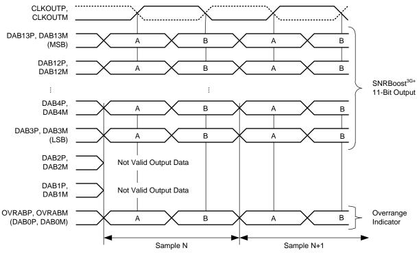
Figure 57. Overrange Indicator (OVR) Timing
