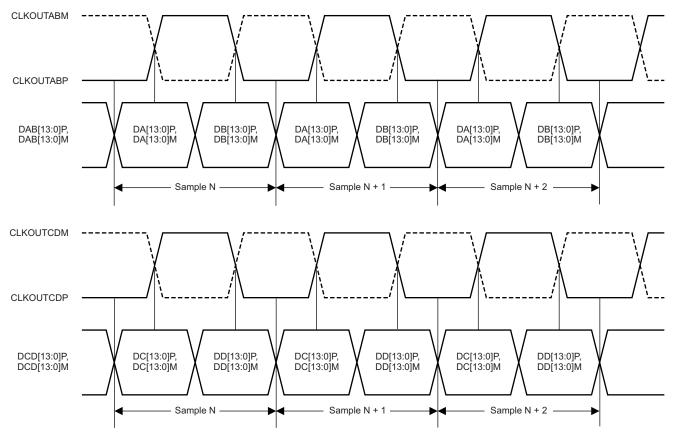
Figure 3. LVDS Output Interface Timing
