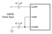
Figure 54. Typical LVCMOS Clock Driving Circuit
