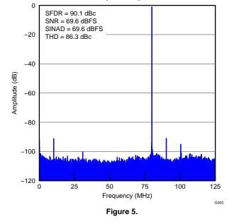
FFT IN 14-BIT MODE INPUT FREQUENCY
