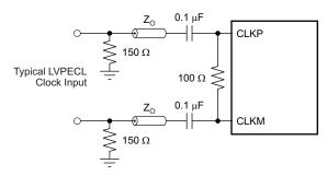
Figure 52. LVPECL Clock Driving Circuit
