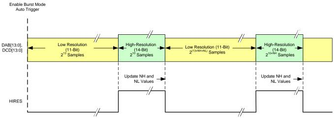
Figure 56. Timing for Auto-Trigger Mode
