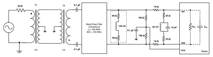
Figure 48. Driving Circuit for a 100- $\Omega$  Source Impedance and Input Frequencies in the Second Nyquist Zone
