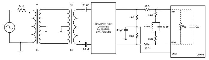
Figure 46. Driving Circuit for a 50- $\Omega$  Source Impedance and Input Frequencies in the Second Nyquist Zone
