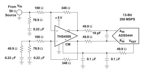
Figure 36. Using the THS4509 With the ADS5444
