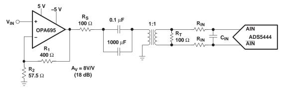
Figure 35. Using the OPA695 With the ADS5444
