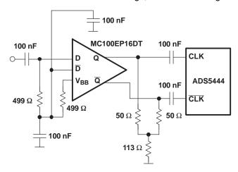
Figure 39. Differential Clock Using PECL Logic
