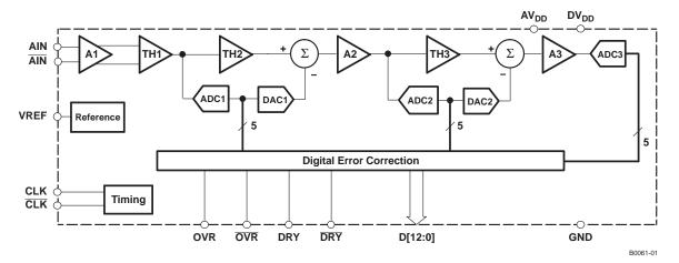
The ADS5444 is available in an 80-pin TQFP PowerPAD™ package. The ADS5444 is built on a state-of-the-art Texas Instruments complementary bipolar process (BiCom3X) and is specified over the full military temperature range (–55°C to 125°C).
