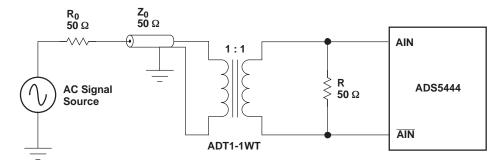
Figure 34. Converting a Single-Ended Input to a Differential Signal Using RF Transformers
