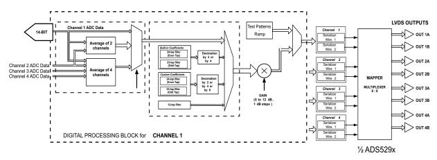
Figure 49. Digital Processing Block Diagram
