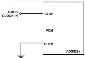
Figure 59. Drive Circuit
