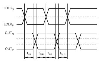
Figure 7. Definition of Setup and Hold Times  $t_{SU} = min(t_{SU1}, t_{SU2})$ ;  $t_H = min(t_{H1}, t_{H2})$
