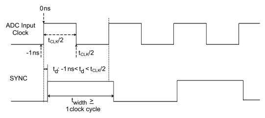
Figure 54. Synchronization Pulse Timing
