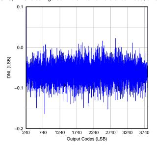
Figure 28. Differential Non-Linearity
