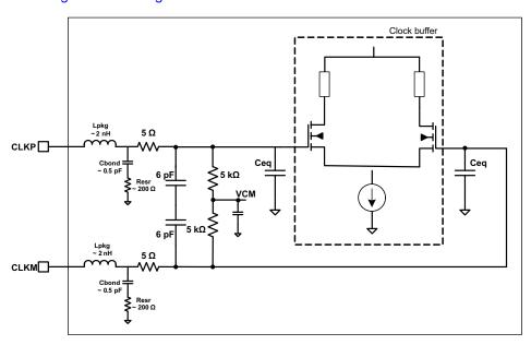
Ceq is approximately 1 to 3 pF, equivalent input capacitance of clock buffer.
