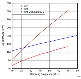
Figure 41. Power Consumption on Digital Supply
