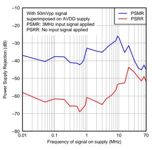
Figure 30. PSRR and PSMR Across Frequency
