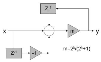
Figure 60. HP Filter Block Diagram
