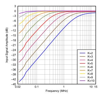
Figure 61. HP Filter Amplitude Response at K = 2 to 10
