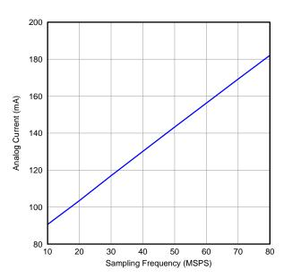
Figure 42. Power Consumption on Analog Supply
