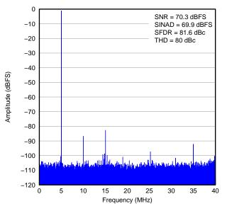
Figure 37. FFT (Full-Band) for 5 MHz Input Signal, Sample Rate = 80 MSPS with Low Frequency Noise Suppression Enabled
