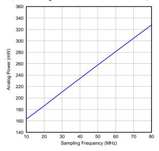
Figure 40. Power Consumption on Analog Supply
