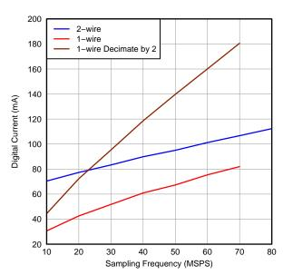
Figure 43. Power Consumption on Digital Supply
