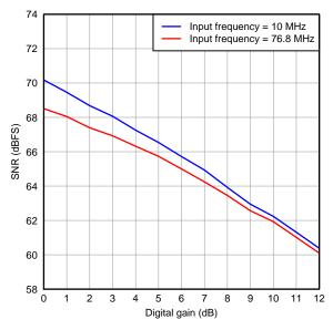
Figure 17. Signal-to-Noise Ratio vs. Digital Gain
