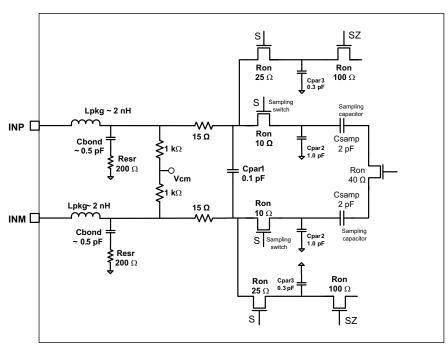
Figure 56. Analog Input Circuit Model
