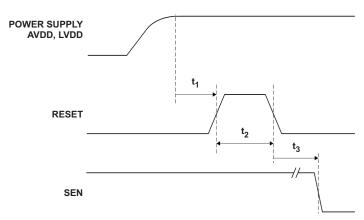
NOTE: A high-going pulse on RESET pin is required in serial interface mode in case of initialization through hardware reset. For parallel interface operation, RESET has to be tied permanently HIGH.
