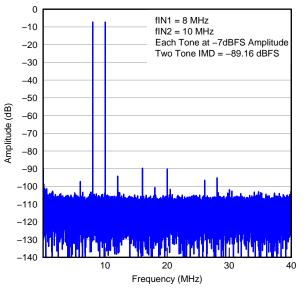
Figure 14. FFT with Two Tone Signal
