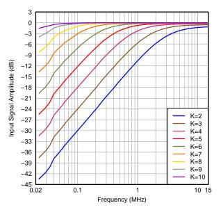
Figure 35. Digital High-Pass Filter Response
