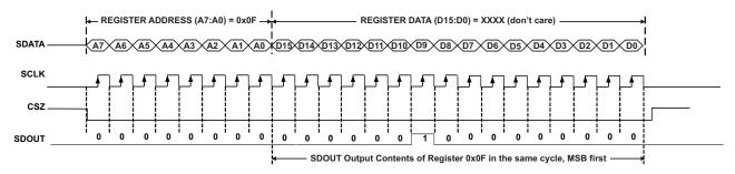
Figure 46. Serial Readout Timing
