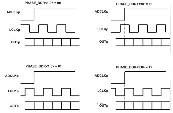
Figure 52. Phase Programmability Modes for LCLK
