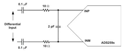
Figure 57. Drive Circuit
