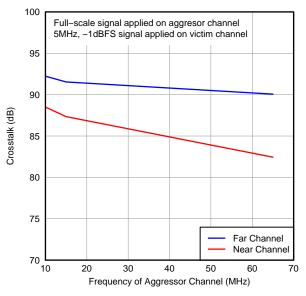
Figure 25. Crosstalk vs. Frequency
