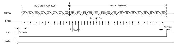
Figure 44. Serial Interface Timing
