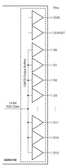
Figure 128. CMOS Output Interface
