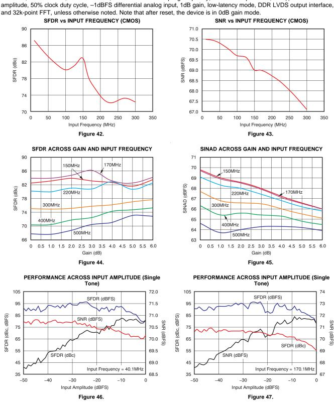
At +25°C, AVDD = 1.8V, DRVDD = 1.8V, maximum rated sampling frequency, sine wave input clock, 1.5V<sub>PP</sub> differential clock amplitude, 50% clock duty cycle, -1dBFS differential analog input, 1dB gain, low-latency mode, DDR LVDS output interface,
