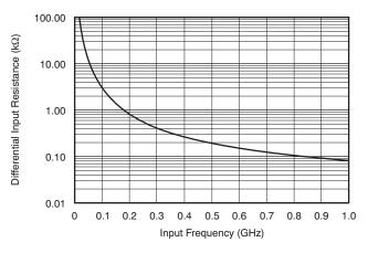
Figure 114. ADC Analog Input Resistance (R<sub>IN</sub>) Across Frequency
