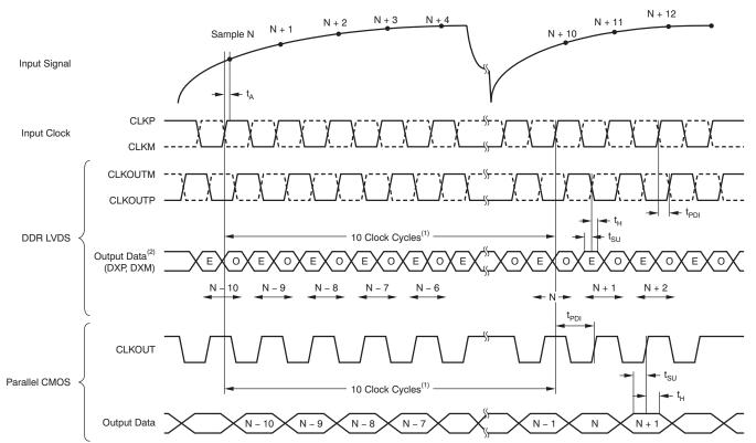
(1) ADC latency in low-latency mode. At higher sampling frequencies,  $t_{DPI}$  is greater than one clock cycle which then makes the overall latency = ADC latency + 1.
