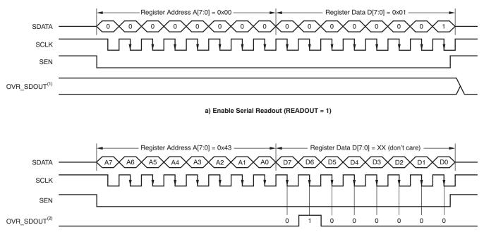
b) Read Contents of Register 0x43. This Register Has Been Initialized with 0x40 (device is put in global power-down mode).
