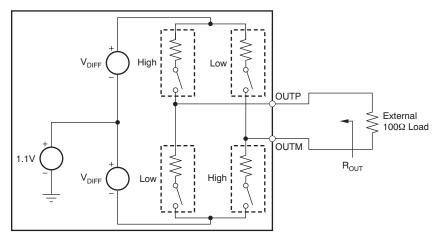
NOTE: Use the default buffer strength to match  $100\Omega$  external termination ( $R_{OUT} = 100\Omega$ ). To match with a  $50\Omega$  external termination, set the LVDS STRENGTH bit ( $R_{OUT} = 50\Omega$ ).
