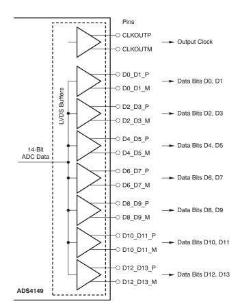
Figure 125. ADS414x LVDS Data Outputs
