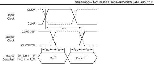
(1) Dn = bits D0, D2, D4, etc. Dn + 1 = Bits D1, D3, D5, etc.
