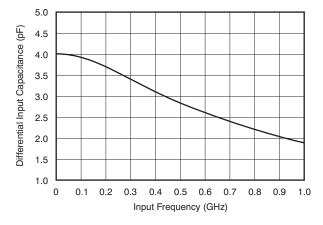
Figure 115. ADC Analog Input Capacitance (C<sub>IN</sub>) Across Frequency
