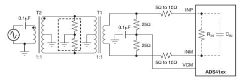
Figure 117. Drive Circuit with High Bandwidth (for High Input Frequencies)
