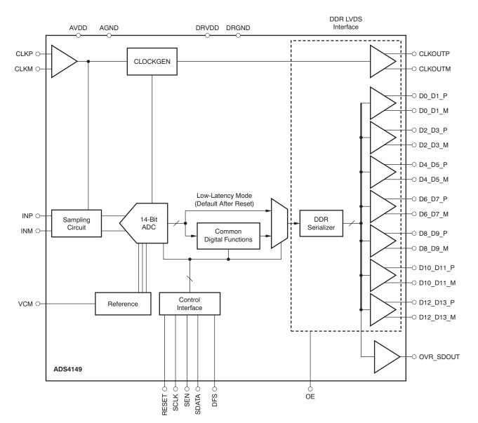
Figure 6. ADS414x Block Diagram
