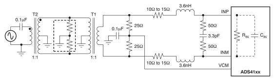
Figure 116. Drive Circuit with Low Bandwidth (for Low Input Frequencies)
