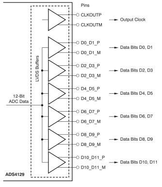
Figure 124. ADS412x LVDS Data Outputs
