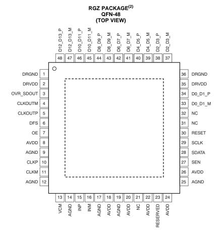
(2) The PowerPAD<sup>™</sup> is connected to DRGND.
