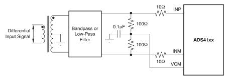
Figure 118. Drive Circuit with 1:4 Transformer
