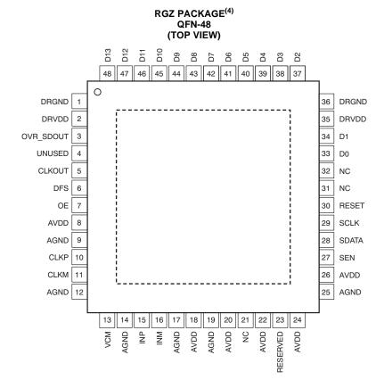
(4) The PowerPAD is connected to DRGND.
