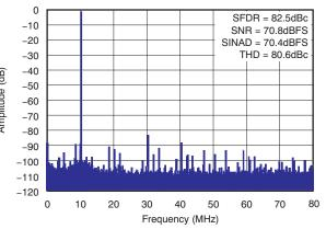
FFT FOR 170MHz INPUT SIGNAL
