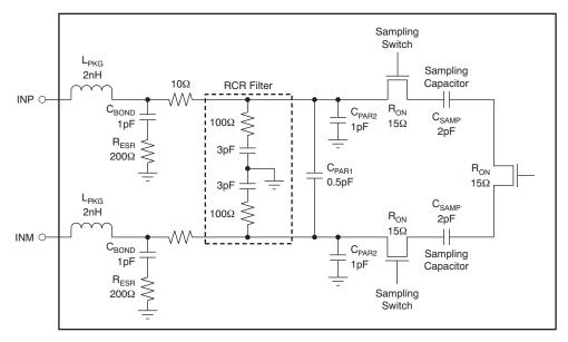
Figure 113. Analog Input Equivalent Circuit
