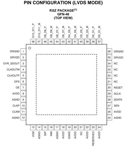
(1) The PowerPAD is connected to DRGND.
