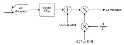
Figure 8-12. Calibration Block Diagram
