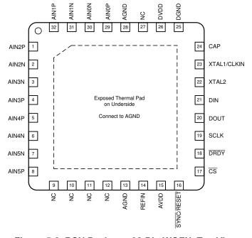
Figure 5-2. RSN Package, 32-Pin WQFN, Top View
