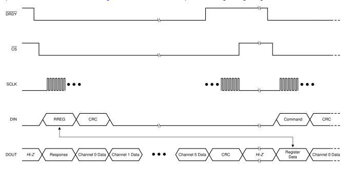
Figure 8-23. Reading a Single Register
