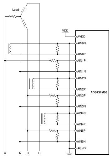
Figure 9-5. Three-Phase Metrology Design Front-End
