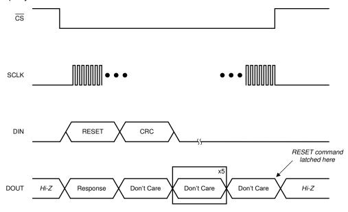
Figure 8-22. RESET Command Frame
