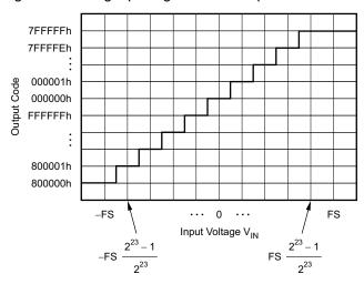
Figure 8-19. Code Transition Diagram
