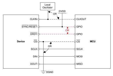
Figure 9-2. Minimum Connections Required to Operate the ADS131M06
