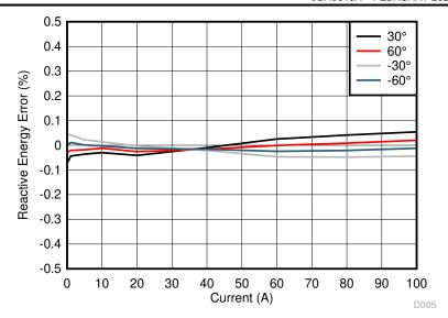
Figure 9-9. Cumulative Reactive Energy % Error Versus Current
