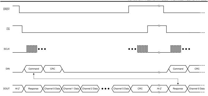
Figure 8-18. Typical Communication Frame
