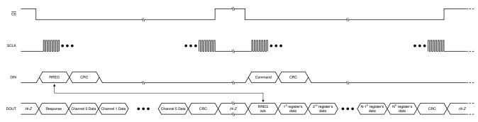
Figure 8-24. Reading Multiple Registers
