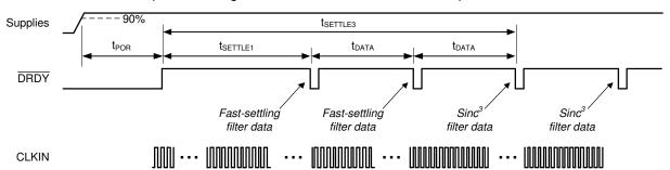
Figure 8-14. Fast Startup Behavior and Settling Times
