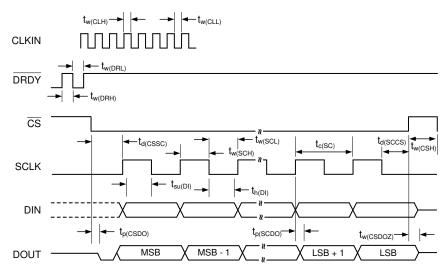
SPI settings are CPOL = 0 and CPHA = 1.  $\overline{\text{CS}}$  transitions must take place when SCLK is low.
