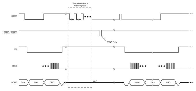
Figure 8-20. Collecting Data After a Pause in Data Collection Using the SYNC/RESET Pin
