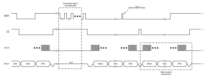
Figure 8-21. Collecting Data After a Pause in Data Collection by Reading Data Twice
