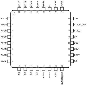
Figure 5-1. PBS Package, 32-Pin TQFP, Top View
