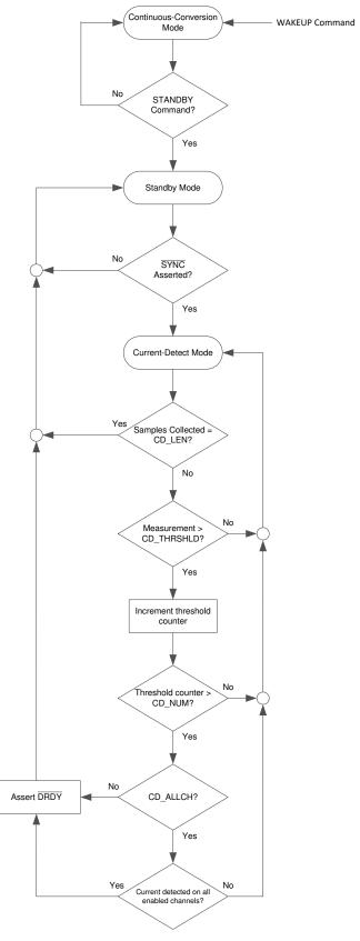
Figure 8-17. Current-Detect Mode Flow Chart
