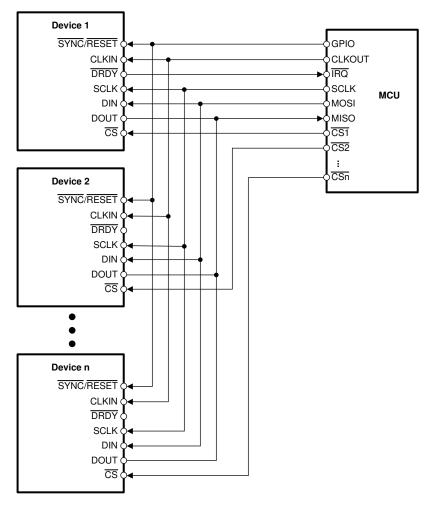
Figure 9-4. Multiple Device Configuration
