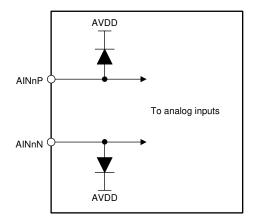
Figure 8-1. Input ESD Protection Circuitry
