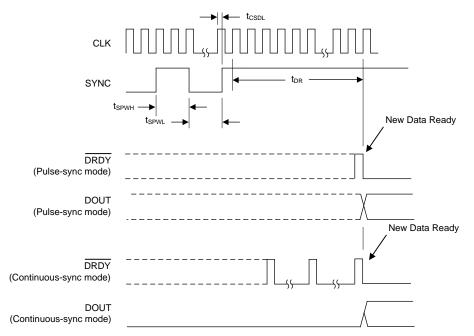
Figure 45. Pulse-Sync and Continuous-Sync Timing With Single Synchronization
