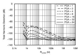
Figure 26. THD vs External Load and Signal Magnitude (PGA); See Figure 27
