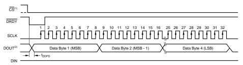
(1) DOUT is in tristate when  $\overline{CS}$  is high.  $\overline{CS}$  can be tied low. See Figure 1 for  $\overline{CS}$  low to valid DOUT propagation time.
