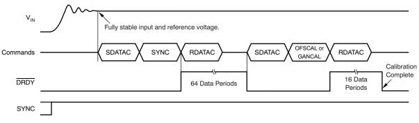
Figure 57. Offset and Gain Calibration Timing
