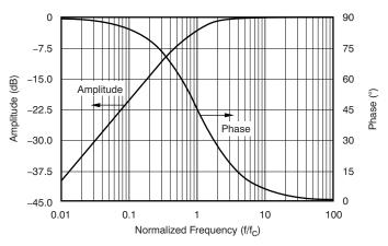
Figure 44. HPF Amplitude and Phase Response
