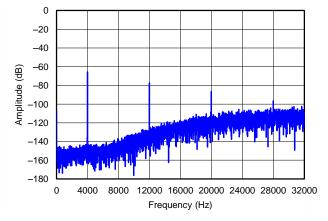
Figure 31. Sinc Output FFT (64 kSPS)
