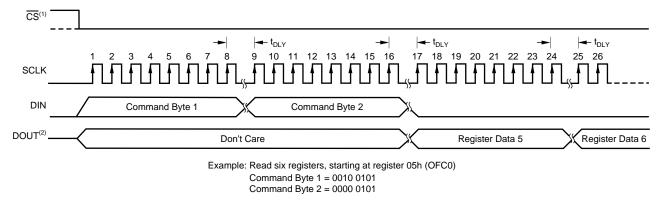
(1) DOUT is in tristate when  $\overline{CS}$  is high.  $\overline{CS}$  can be tied low. See Figure 1 for  $\overline{CS}$  low to SCLK rising edge time.
