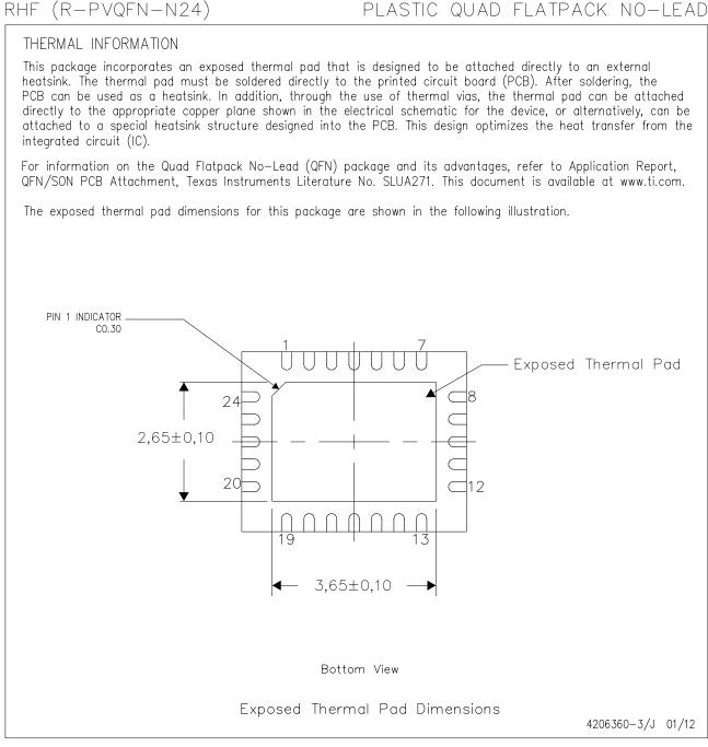
NOTE: All linear dimensions are in millimeters
