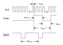
Figure 46. Continuous-Sync Timing With SYNC Clock
