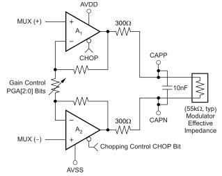
(1) Modulator input impedance scales with clock rate.
