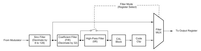
Figure 35. Digital Filter and Output Code Processing
