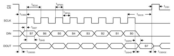
Figure 1. Serial Interface Timing Diagram
