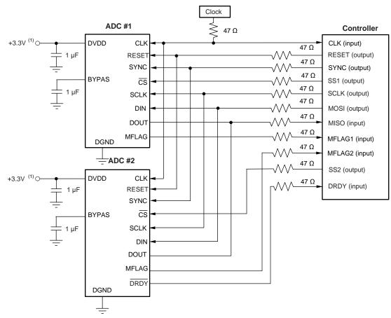
(1) For DVDD < 2.25 V, tie DVDD and BYPASS together. see the DVDD Power Supply section.
