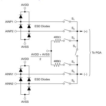
Figure 25. Analog Inputs and Multiplexer
