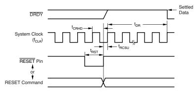
Figure 47. Reset Timing
