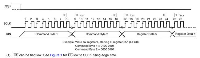
Figure 61. Write Register Data (Table 24 shows t<sub>DLY</sub>)
