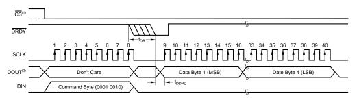
(1) DOUT is in tristate when  $\overline{CS}$  is high.  $\overline{CS}$  can be tied low. See Figure 1 for  $\overline{CS}$  low to SCLK rising edge time.
