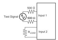
Figure 27. Driving an External Load Through the Multiplexer
