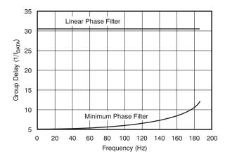
Figure 42. FIR Group Delay (f<sub>DATA</sub> = 500Hz)
