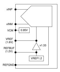
Figure 8-15. Different voltage reference options for ADC368x
