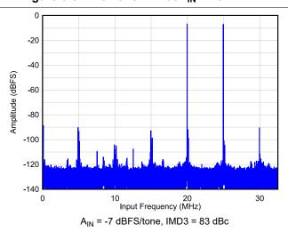
Figure 6-10. Two Tone FFT at  $F_{IN} = 40/45 \text{ MHz}$
