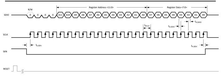
Figure 8-42. Serial Register Write Timing Diagram
