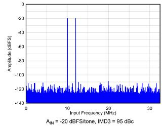
Figure 6-9. Two Tone FFT at  $F_{IN}$  = 10/12 MHz
