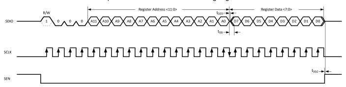
Figure 8-43. Serial Register Read Timing Diagram
