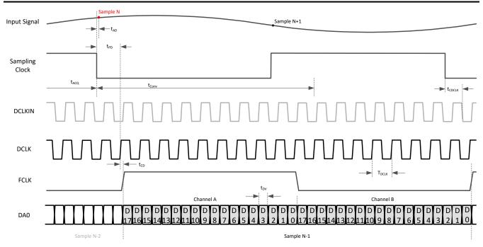
Figure 7-3. Timing diagram: 1/2-wire SLVDS
