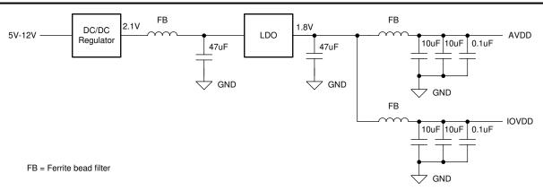
Figure 10-2. Example: LDO Linear Regulator Approach
