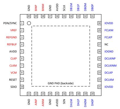
Figure 5-1. RSB Package, 40-Pin WQFN, Top View
