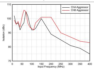
Figure 6-20. Isolation vs Input Frequency
