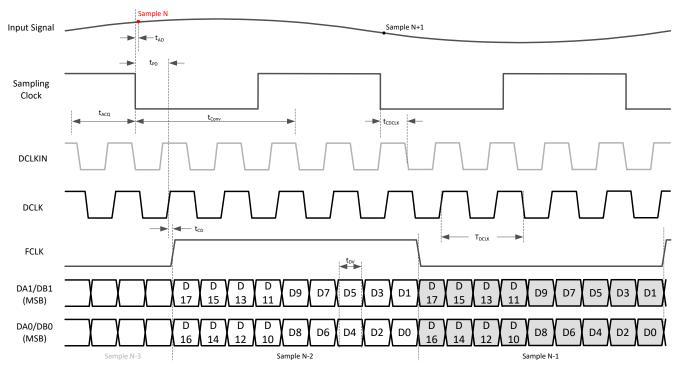
Figure 7-1. Timing diagram: 2-wire SLVDS
