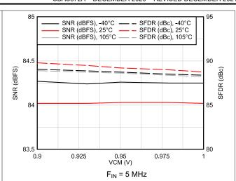
Figure 6-18. AC Performance vs VCM vs Temperature
