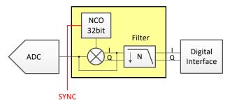
Figure 8-19. Internal Digital Decimation Filter
