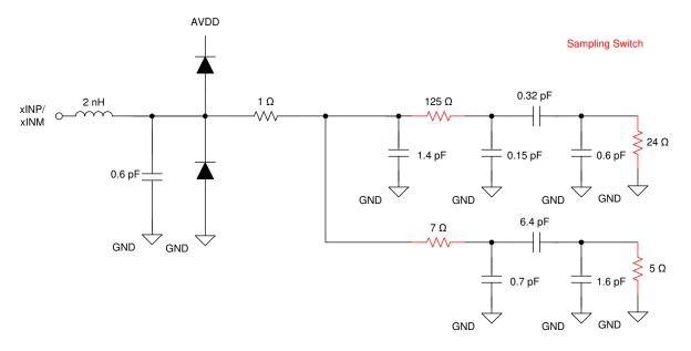
Figure 8-1. Equivalent input network
