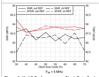
Figure 6-19. AC Performance vs Clock Duty Cycle
