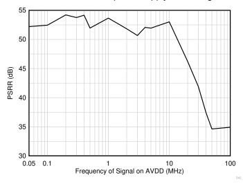
Figure 10-1. Power supply rejection ratio (PSRR) vs frequency
