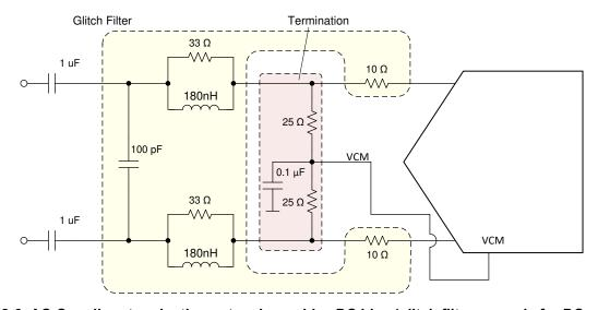
Figure 8-6. AC-Coupling: termination network provides DC bias (glitch filter example for DC - 30 MHz)
