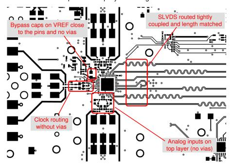
Figure 11-1. Layout example: top layer of ADC368x EVM
