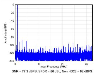
Figure 6-6. Single Tone FFT at F<sub>IN</sub> = 64 MHz
