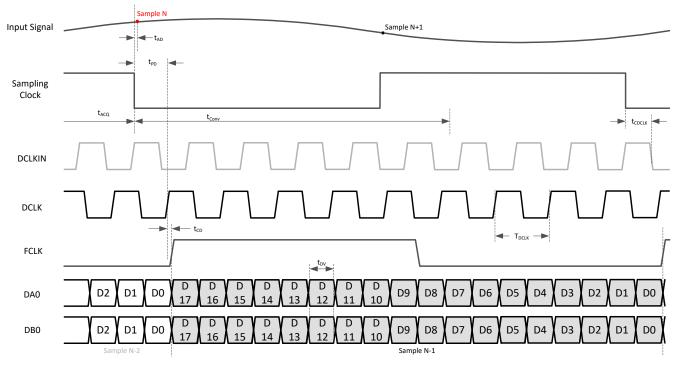
Figure 7-2. Timing diagram: 1-wire SLVDS
