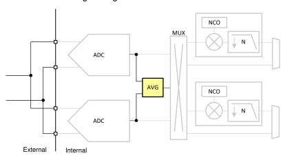
Figure 8-40. Digital Channel Averaging Diagram
