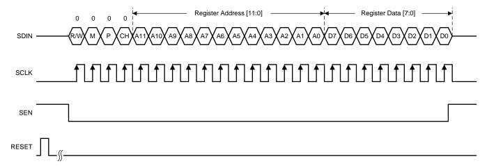
Figure 115. SPI Write Timing Diagram for the Analog Bank
