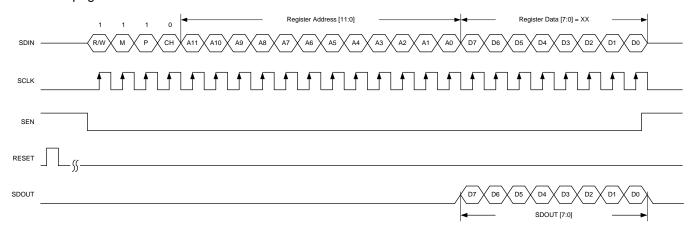
Figure 119. SPI Read Timing Diagram for the Digital Bank
