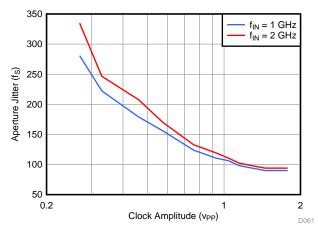
Figure 66. Equivalent Aperture Jitter vs Input Clock Amplitude
