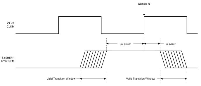
Figure 2. SYSREF Timing Diagram
