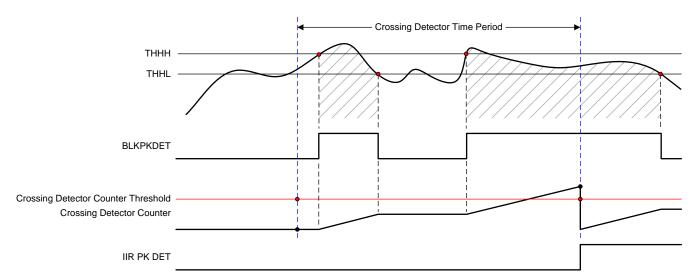
Figure 106. Crossing Detector Timing Diagram
