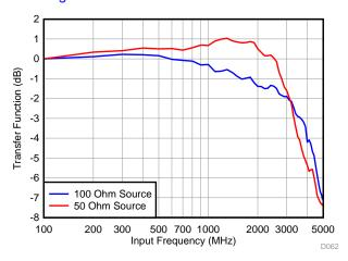
Figure 62. Input Bandwidth with a 100- $\Omega$  Source Resistance
