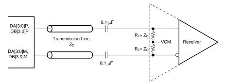
Figure 100. External Serial JESD204B Interface Connection
