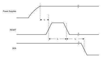
Figure 231. Hardware Reset Timing Diagram
