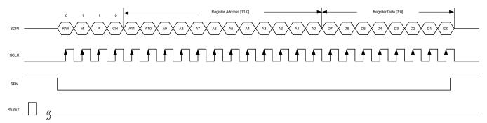
Figure 118. SPI Write Timing Diagram for Digital Bank Register Write
