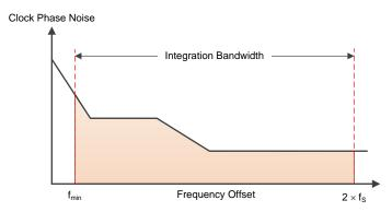
Figure 233. Integration Bandwidth for Extracting Jitter from Clock Phase Noise
