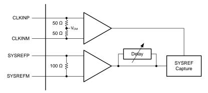
Figure 67. SYSREF Internal Circuit Diagram
