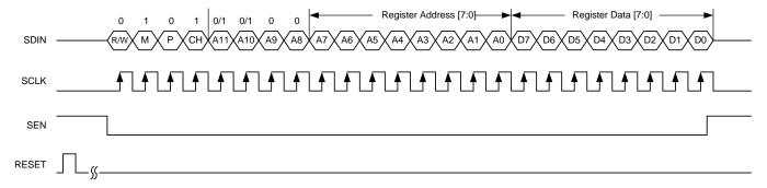
Figure 120. SPI Write Timing Diagram for the Decimation and Power Detector Pages
