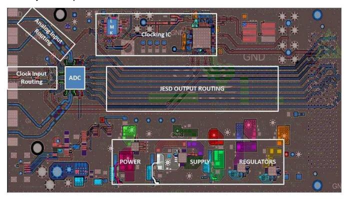
Figure 244. ADC32RF44EVM Layout
