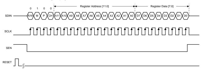
Figure 117. SPI Write Timing Diagram for Digital Bank Page Selection
