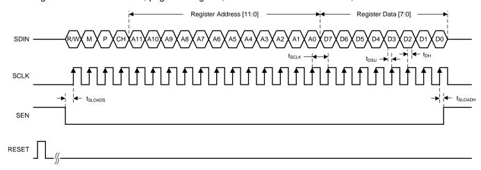
Figure 113. SPI Timing Diagram
