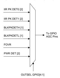
Figure 108. GPIO Output MUX Implementation
