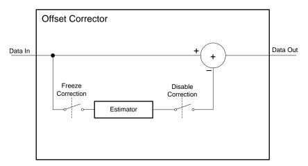
Figure 236. Offset Corrector in the ADC32RF44
