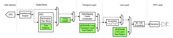
Figure 109. Test Pattern Generator Implementation
