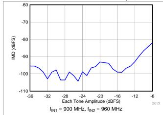
Figure 15. Intermodulation Distortion vs Input Amplitude (900 MHz and 960 MHz)
