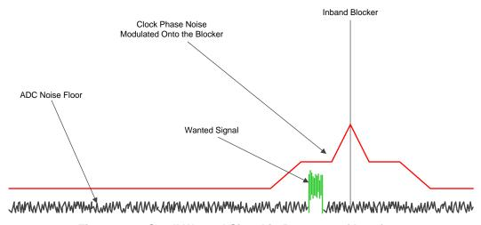
Figure 234. Small Wanted Signal in Presence of Interferer
