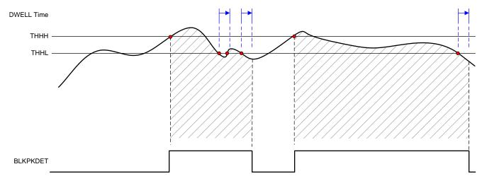
Figure 104. Peak Power Detector Timing Diagram
