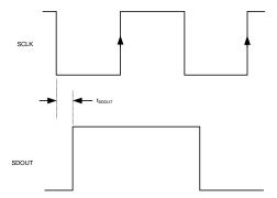
Figure 114. SDOUT Timing
