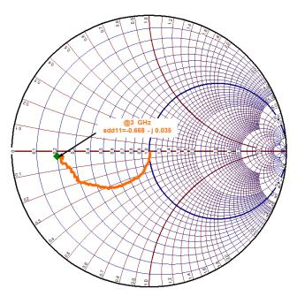
Figure 65. SDD11 of the Clock Input
