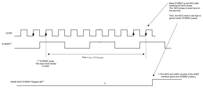
t<sub>SYSREF</sub> is a period of the SYSREF waveform.
