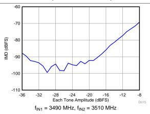
Figure 17. Intermodulation Distortion vs Input Amplitude (3490 MHz and 3510 MHz)
