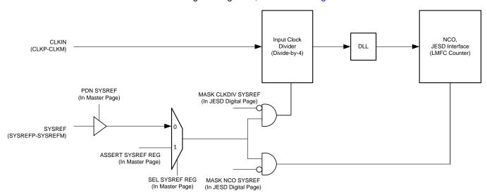
Figure 68. Using SYSREF to Reset the Clock Divider, the NCO, and the LMFC Counter
