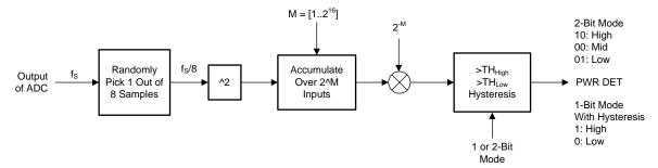
Figure 107. RMS Power Detector Implementation
