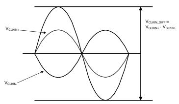
Figure 57. Input Clock Diagram
