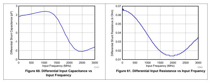
Each input pin (INP, INM) must swing symmetrically between (CM + 0.3375 V) and (CM - 0.3375 V), resulting in a 1.35-V<sub>PP</sub> (default) differential input swing. The input sampling circuit has a 3-dB bandwidth that extends up to approximately 3.2 GHz, as shown in Figure 62.
