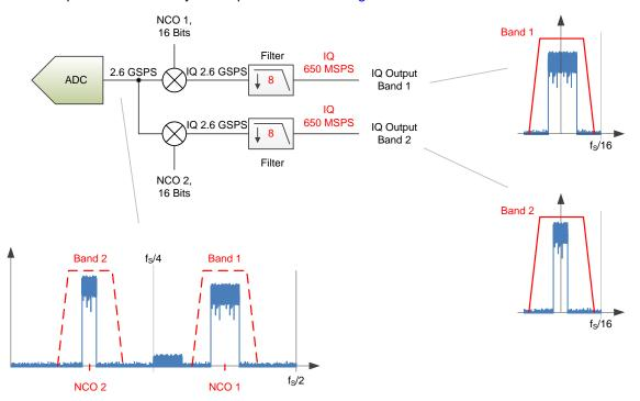
Figure 74. Dual-Band Example
