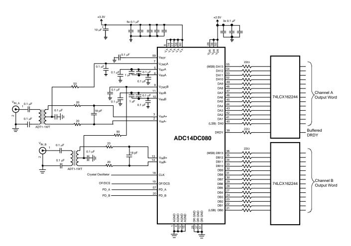
Figure 21. Application Circuit
