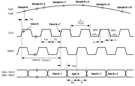
Figure 1. Output Timing
