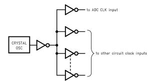
Figure 22. Isolating the ADC Clock from other Circuitry with a Clock Tree
