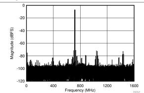
DES\_EN = 0, FG calibration,  $f_S$  = 3200 MSPS,  $f_1$  = 2483 MHz,  $f_2$  = 2493 MHz,  $A_{\text{IN}}$  = -7 dBFS per tone, SFDR = -71 dBFS, IMD3 = -71 dBFS, IMD2 = -75 dBFS
