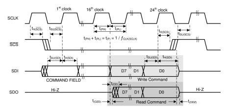
Figure 9. Serial Interface Timing
