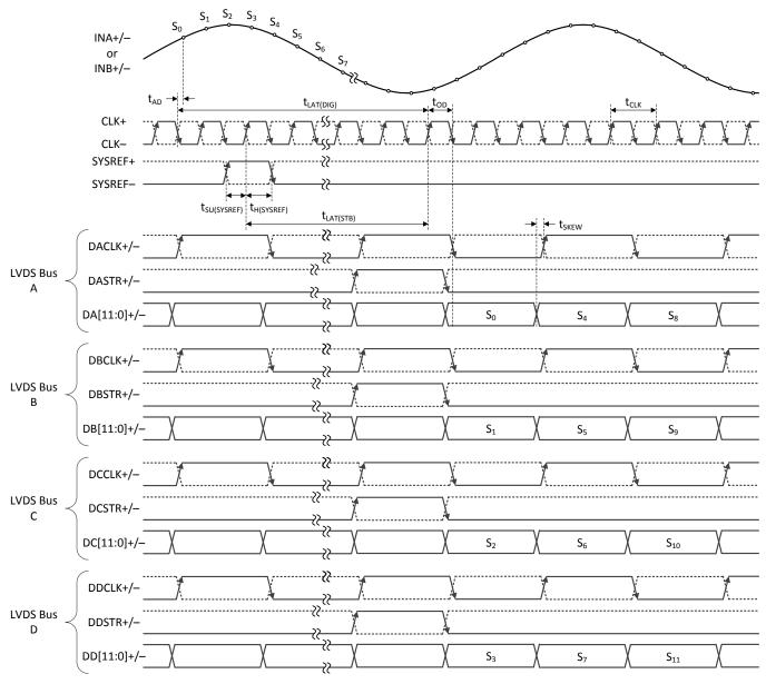
Figure 7. Single-Channel, 4-Bus, Aligned-Mode Timing (LDEMUX = 1, DES\_EN = 1, LALIGNED = 1)
