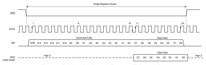
Figure 82. Serial Interface Protocol: Single Read/Write Operation
