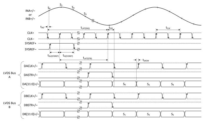
Figure 5. Single-Channel, 2-Bus, Aligned-Mode Timing (LDEMUX = 0, DES\_EN = 1, LALIGNED = 1)
