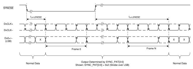
Figure 8. SYNCSE Timing Diagram
