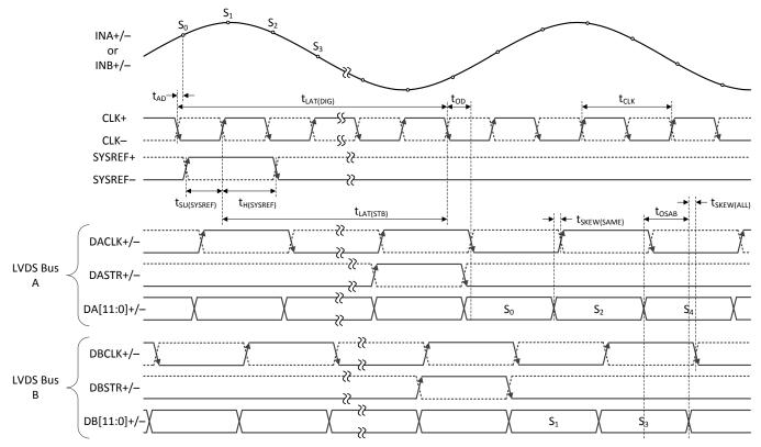
Figure 4. Single-Channel, 2-Bus, Staggered-Mode Timing (LDEMUX = 0, DES\_EN = 1, LALIGNED = 0)
