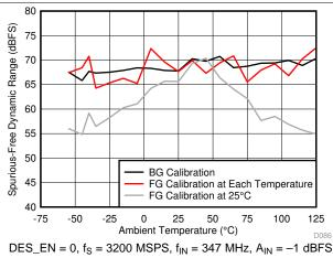
Figure 62. SFDR vs Temperature and Calibration Mode
