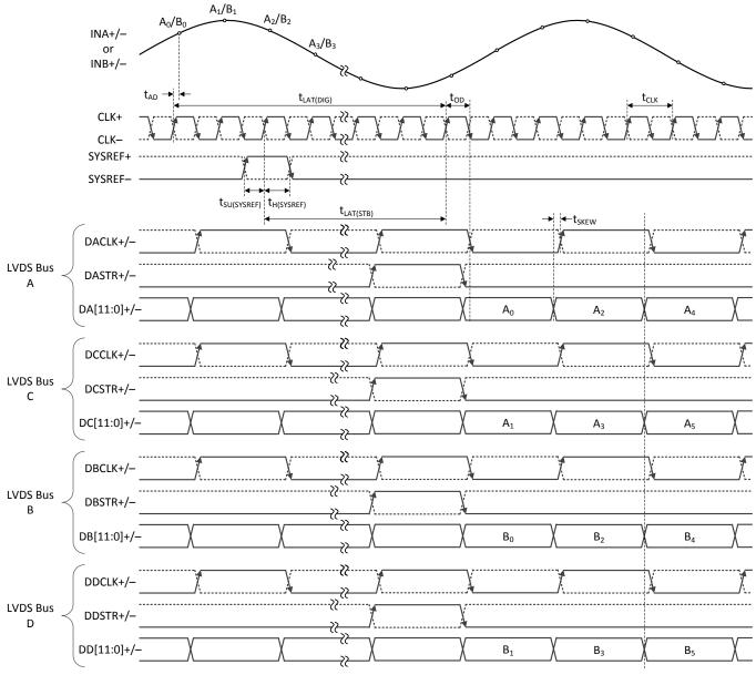
Figure 3. Dual-Channel, 4-Bus, Aligned-Mode Timing (LDEMUX = 1, DES\_EN = 0, LALIGNED = 1)
