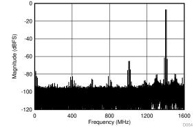
DES\_EN = 0, FG calibration,  $f_S$  = 3200 MSPS,  $f_1$  = 4992 MHz,  $f_2$  = 5002 MHz,  $A_{IN}$  = -7 dBFS per tone, SFDR = -61 dBFS, IMD3 = -61 dBFS, IMD2 = -77 dBFS
