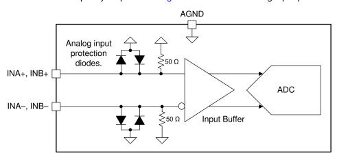
Figure 78. ADC12DL3200 Analog Input Internal Termination
