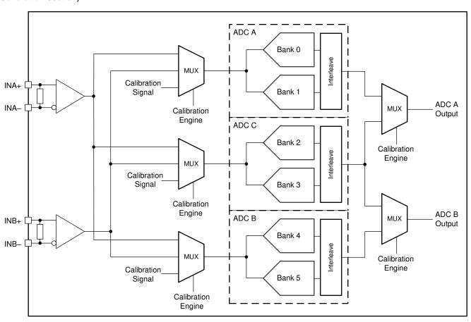
Figure 81. ADC12DL3200 Calibration System Block Diagram
