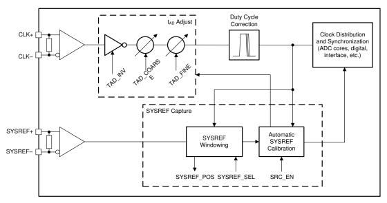
Figure 79. ADC12DL3200 Clocking Subsystem
