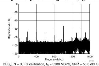
Figure 44. Single-Tone FFT at  $f_{IN}$  = 8197 MHz,  $A_{IN}$  = -1 dBFS
