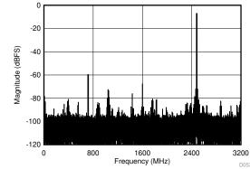
DES\_EN = 1, FG calibration,  $f_S$  = 6400 MSPS,  $f_1$  = 2483 MHz,  $f_2$  = 2493 MHz,  $A_{IN}$  = -7 dBFS per tone, SFDR = -60 dBFS, IMD3 = -72 dBFS, IMD2 = -78 dBFS
