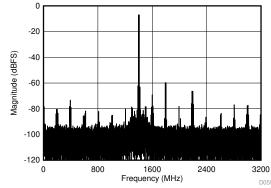
DES\_EN = 1, FG calibration,  $f_S$  = 6400 MSPS,  $f_1$  = 4992 MHz,  $f_2$  = 5002 MHz,  $A_{IN}$  = -7 dBFS per tone, SFDR = -60 dBFS, IMD3 = -62 dBFS, IMD2 = -78 dBFS
