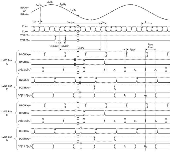
Figure 2. Dual-Channel, 4-Bus, Staggered-Mode Timing (LDEMUX = 1, DES\_EN = 0, LALIGNED = 0)
