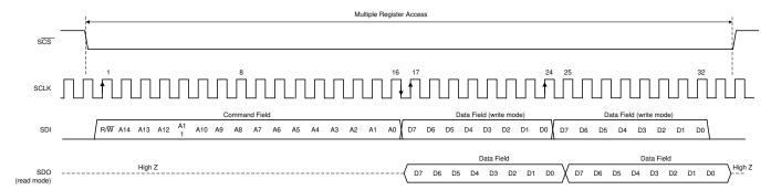
Figure 83. Serial Interface Protocol: Streaming Read/Write Operation
