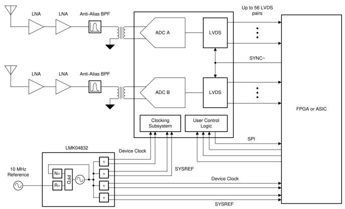
Figure 168. Typical Configuration for Wideband RF Sampling
