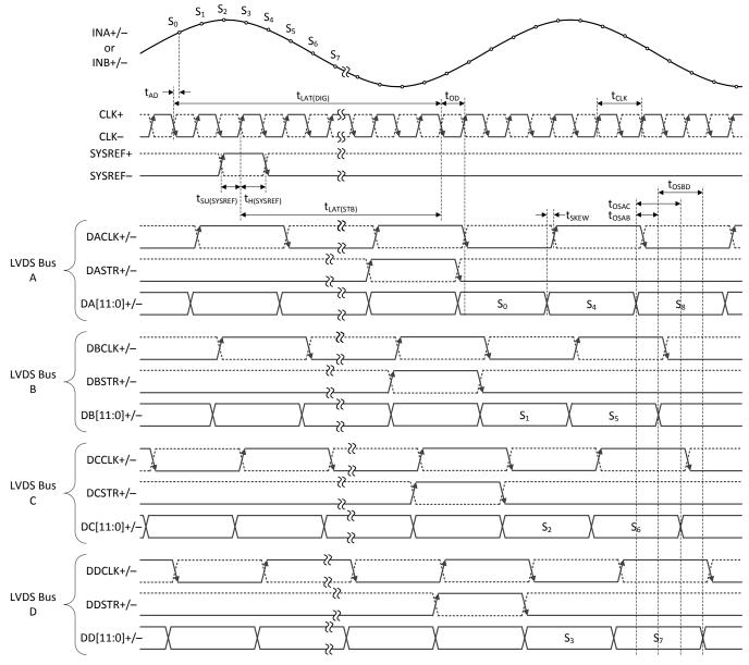
Figure 6. Single-Channel, 4-Bus, Staggered-Mode Timing (LDEMUX = 1, DES\_EN = 1, LALIGNED = 0)
