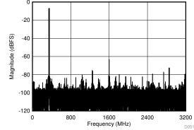
DES\_EN = 1, FG calibration,  $f_S$  = 6400 MSPS,  $f_1$  = 342 MHz,  $f_2$  = 352 MHz,  $A_{IN}$  = -7 dBFS per tone, SFDR = -73 dBFS, IMD3 = -81 dBFS, IMD2 = -88 dBFS
