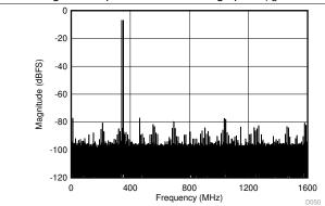
DES\_EN = 0, FG calibration,  $f_S$  = 3200 MSPS,  $f_1$  = 342 MHz,  $f_2$  = 352 MHz,  $A_{IN}$  = -7 dBFS per tone, SFDR = -77 dBFS, IMD3 = -87 dBFS, IMD2 = -77 dBFS
