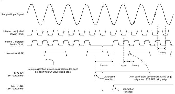
Figure 80. SYSREF Calibration Timing Diagram
