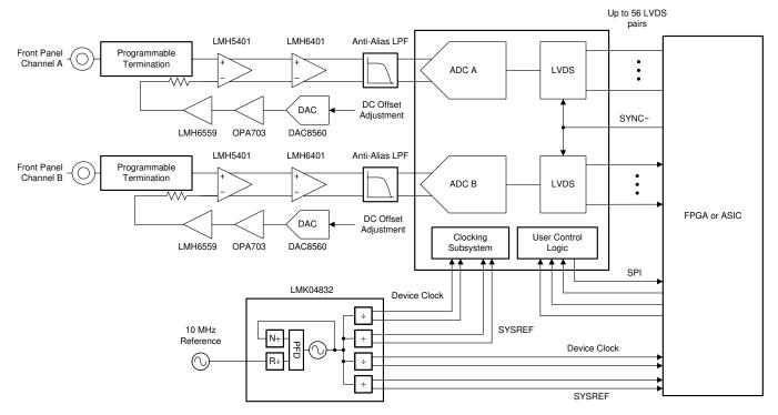
Figure 171. Typical Configuration for a Reconfigurable Oscilloscope
