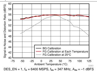
Figure 58. SINAD vs Temperature and Calibration Mode
