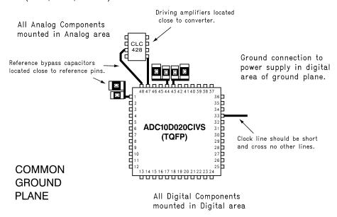
Figure 68. An Acceptable Layout Pattern
