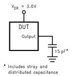
Figure 5. AC Test Circuit
