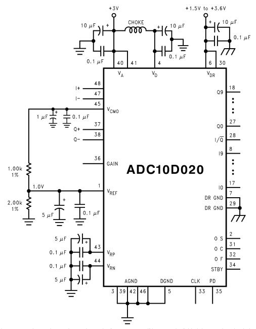
The  $V_{CMO}$  output pin may be used as an internal reference source if its output is divided down and not loaded excessively.
