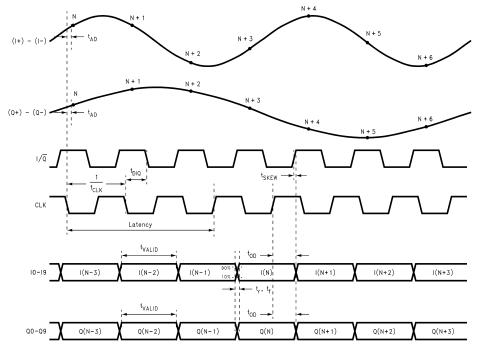
Figure 4. ADC10D020 Timing Diagram for Parallel Mode
