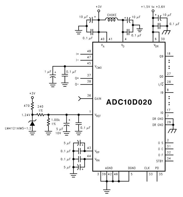
Figure 66. Setting An Accurate Reference Voltage
