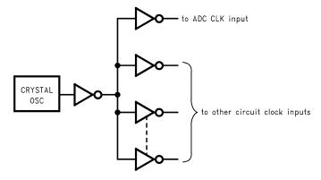
Figure 69. Isolating the ADC Clock from Digital Circuitry
