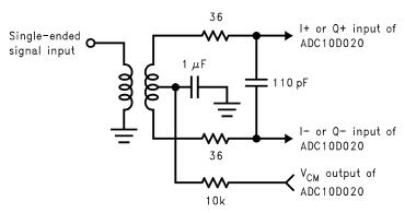
Use of an input transformer for single-ended to differential conversion can simplify circuit design for single-ended signals.
