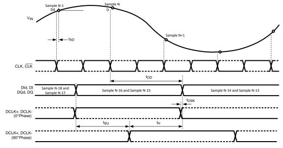
Figure 4. ADC08D500 Timing — DDR Clocking
