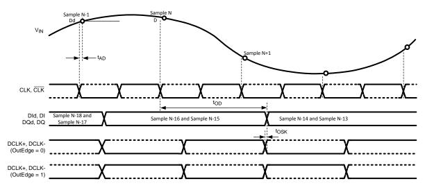
Figure 3. ADC08D500 Timing — SDR Clocking
