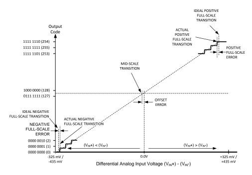
Figure 2. Input / Output Transfer Characteristic
