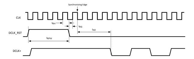
Figure 6. Clock Reset Timing in DDR Mode
