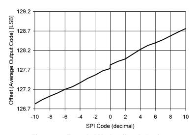
Figure 30. Extended Mode Offset Behavior
