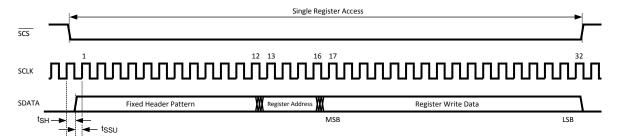
Figure 5. Serial Interface Timing
