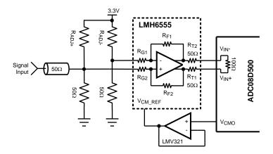
Figure 32. Example of Servoing the Analog Input with  $V_{\text{CMO}}$
