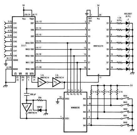
Note: DUT pin numbers in parentheses are for ADC0844, others are for ADC0848.
