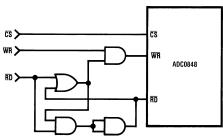
$\overline{\text{CS}} \cdot \overline{\text{WR}}$  will update the channel configuration and start a conversion.  $\overline{\text{CS}} \cdot \overline{\text{RD}}$  will read the conversion data and start a new conversion without updating the channel configuration. Waiting for the end of this conversion is not necessary. A  $\overline{\text{CS}} \cdot \overline{\text{WR}}$  can immediately follow the  $\overline{\text{CS}} \cdot \overline{\text{RD}}$ .
