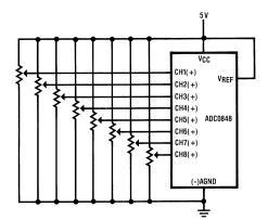
Figure 13. Referencing Examples - Ratiometric
