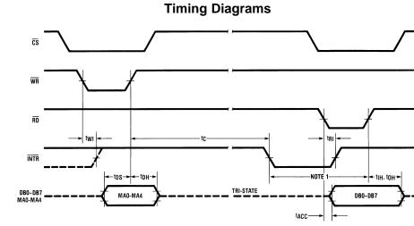
Read strobe must occur at least 600 ns after the assertion of interrupt to ensure reset of  $\overline{\rm INTR}$  . MA stands for MUX address.
