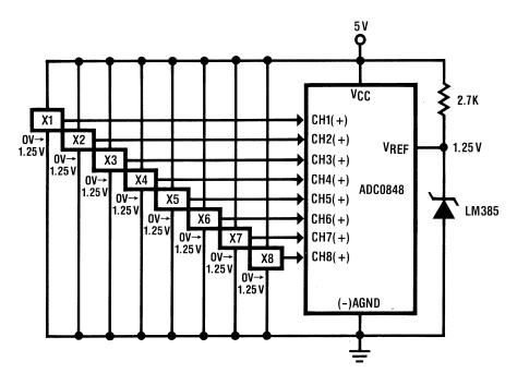
Figure 14. Referencing Examples - Absolute with a Reduced Span
