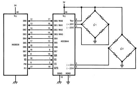
Figure 23. ADC0844—INS8039 Interface
