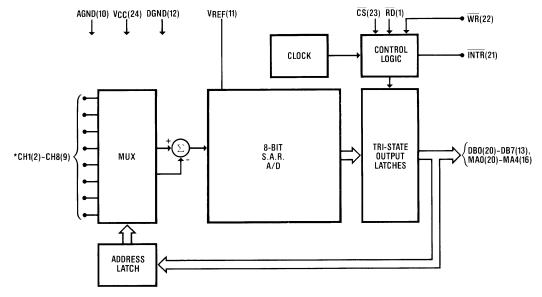
\* ADC0848 shown in PDIP Package CH5-CH8 not included on the ADC0844
