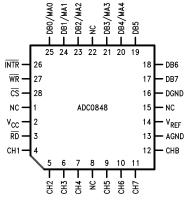
Figure 1. PLCC Package (Top View)
