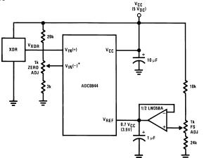
Figure 20. Operating with Automotive Ratiometric Transducers
