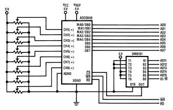
Figure 24. I/O Interface to NSC800
