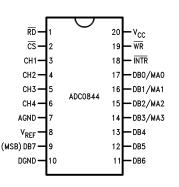
Figure 2. 20-Pin PDIP (Top View)
