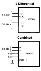
Figure 12. Analog Input Multiplexer Options
