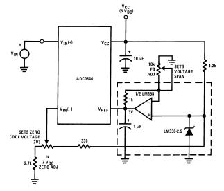
Figure 15. Zero-Shift and Span Adjust ( $2V \le V_{IN} \le 5V$ )
