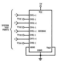
Figure 19. High Accuracy Comparators
