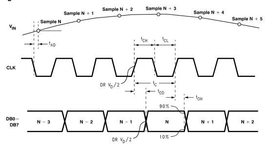
Figure 1. ADC08100 Timing Diagram
