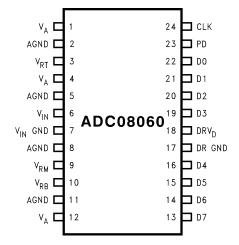
Figure 1. 24-Lead TSSOP See PW Package
