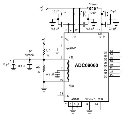
Because of the ladder and external resistor tolerances, the reference voltage can vary too much for some applications.
