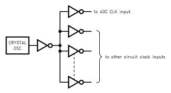
Figure 34. Isolating the ADC Clock from Digital Circuitry
