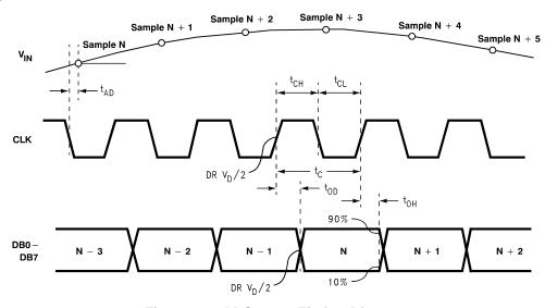
Figure 29. ADC08060 Timing Diagram
