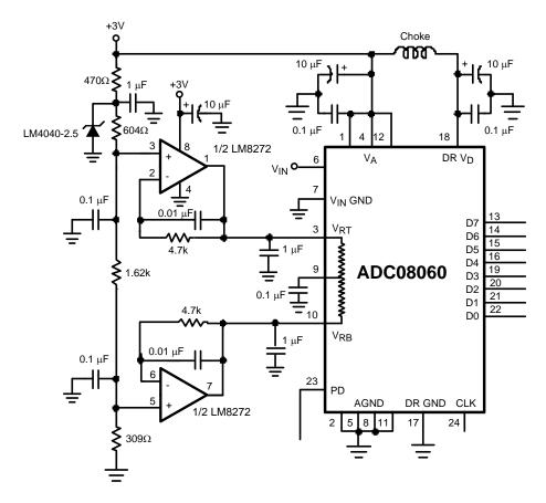
Driving the reference to force desired values requires driving with a low impedance source.
