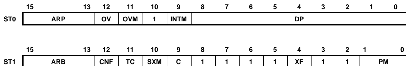
Figure 10. Status and Control Register Organization
