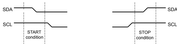
Figure 15-3. START and STOP Conditions
