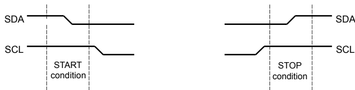
Figure 15-3. START and STOP Conditions
