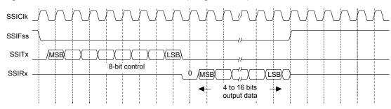
Figure 11-10. MICROWIRE Frame Format (Single Frame)
