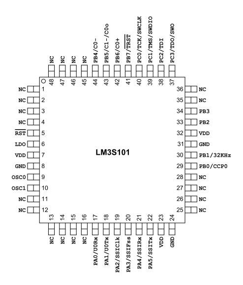
Figure 13-3. 48-Pin QFN Package Pin Diagram<sup>1</sup>
