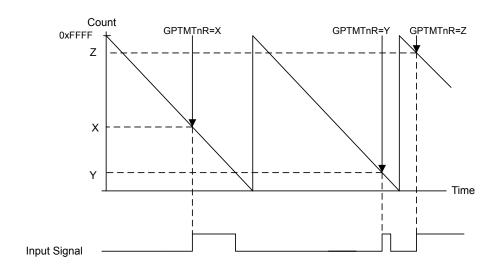
Figure 8-3. 16-Bit Input Edge Time Mode Example
