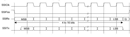
Figure 11-4. Freescale SPI Format (Single Transfer) with SPO=0 and SPH=0
