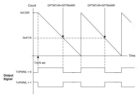
Figure 8-4. 16-Bit PWM Mode Example
