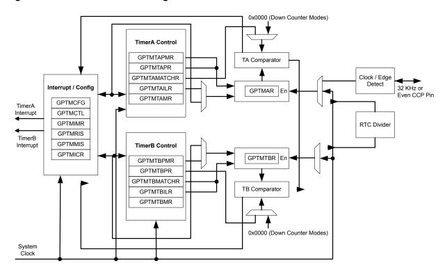
Figure 8-1. GPTM Module Block Diagram
