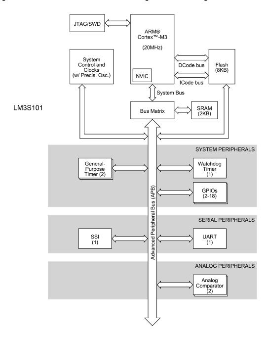
Figure 1-1. Stellaris LM3S101 Microcontroller High-Level Block Diagram
