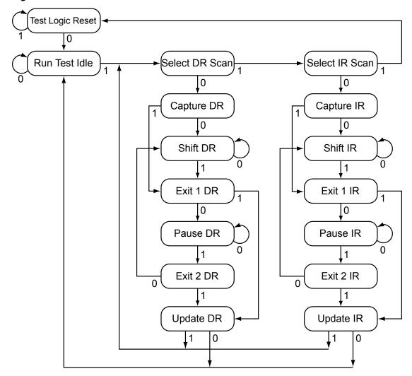
Figure 4-2. Test Access Port State Machine
