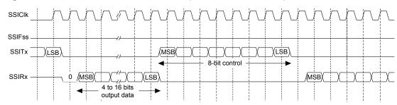
Figure 11-11. MICROWIRE Frame Format (Continuous Transfer)
