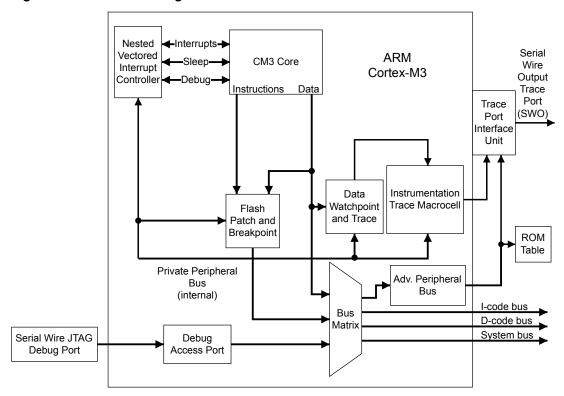
Figure 2-1. CPU Block Diagram
