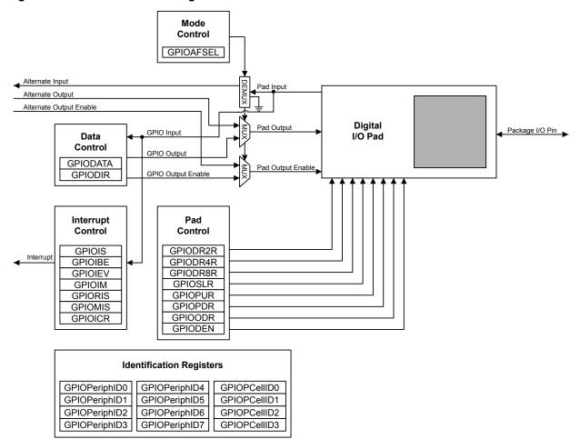
Figure 7-2. GPIO Port Block Diagram
