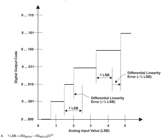
Figure 7-13. Differential Nonlinearity (DNL) Error<sup>(A)</sup>
