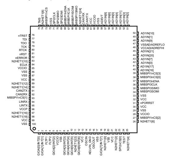
Figure 4-2. PZ QFP Package Pinout (100-Pin)
