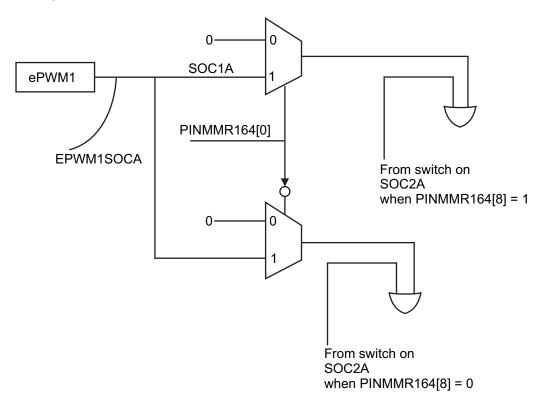
Figure 7-11. ePWM1SOC1A Switch Implementation
