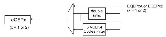
Figure 7-9, eQEPx Input Synchronization Selection Detail
