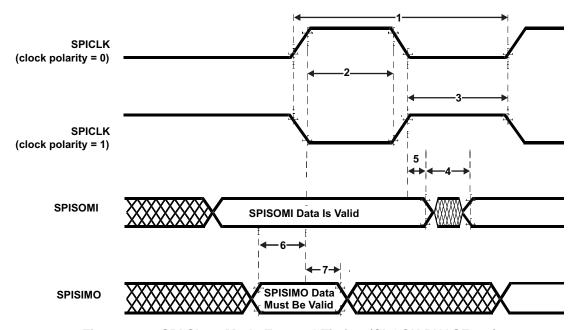
Figure 7-26. SPI Slave Mode External Timing (CLOCK PHASE = 1)
