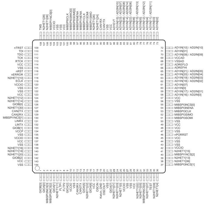
A. Pins can have multiplexed functions. Only the default function is shown in Figure 4-1.
