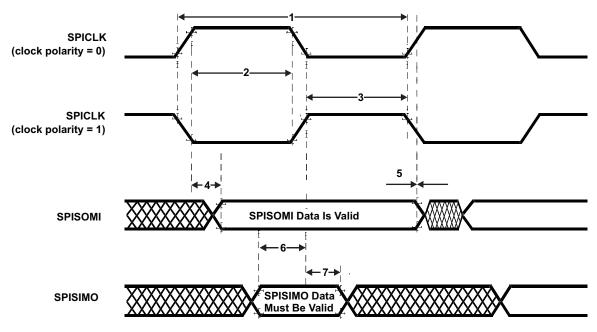
Figure 7-24. SPI Slave Mode External Timing (CLOCK PHASE = 0)
