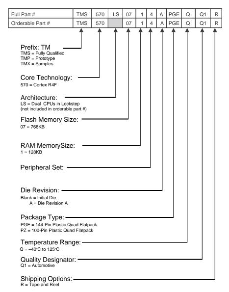
Figure 9-1. TMS570LS0714 Device Numbering Conventions
