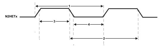
Figure 7-16. N2HET Input Capture Timings
