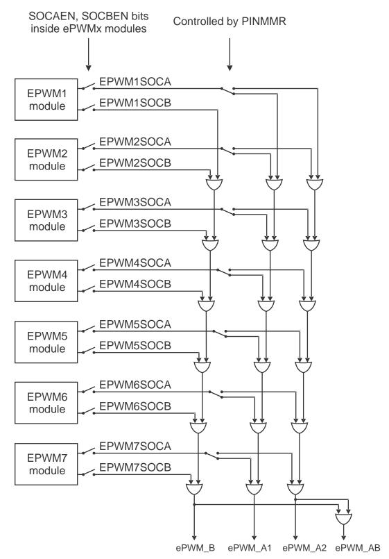
Figure 7-10. ADC Trigger Source Generation from ePWMx
