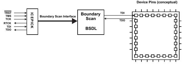
Figure 6-17. Boundary Scan Implementation (Conceptual Diagram)
