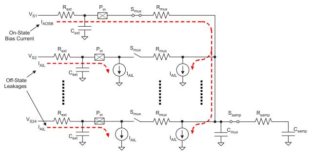
Figure 7-12. MibADC Input Equivalent Circuit
