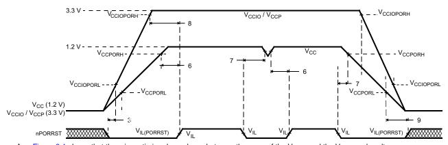
A. Figure 6-1 shows that there is no timing dependency between the ramp of the  $V_{CCIO}$  and the  $V_{CC}$  supply voltages.
