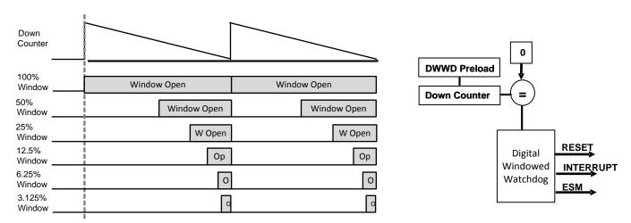
Figure 6-13. Digital Windowed Watchdog Example
