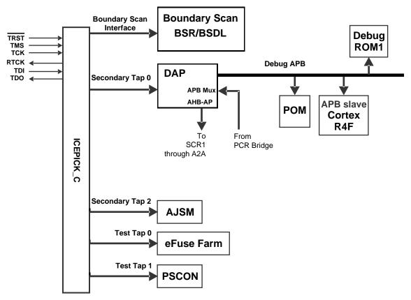
Figure 6-14. Debug Subsystem Block Diagram
