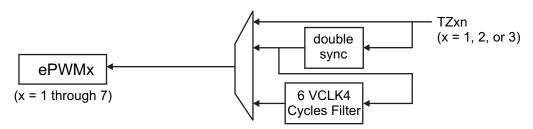
Figure 7-4. ePWMx Input Synchronization Selection Detail
