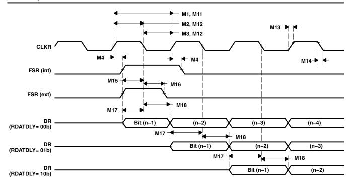
Figure 6-40. McBSP Receive Timing
