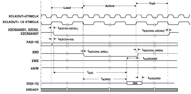
NOTES: A. All XINTF accesses (lead period) begin on the rising edge of XCLKOUT. When necessary, the device inserts an alignment cycle before an access to meet this requirement.
