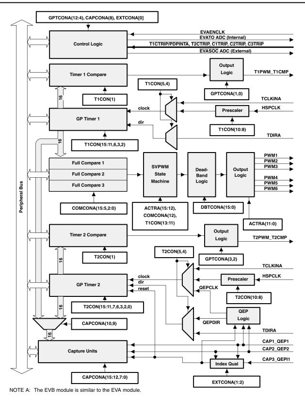
Figure 4–3. Event Manager A Functional Block Diagram (See Note A)
