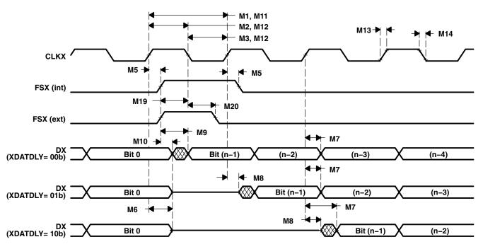
Figure 6-41. McBSP Transmit Timing
