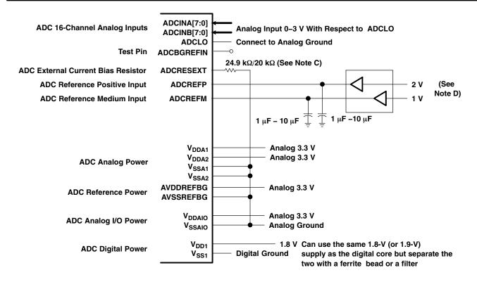
NOTES: A. External decoupling capacitors are recommended on all power pins.
