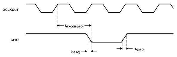
Figure 6-20. General-Purpose Output Timing
