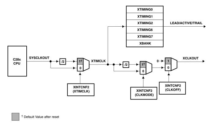
Figure 6-27. Relationship Between XTIMCLK and SYSCLKOUT
