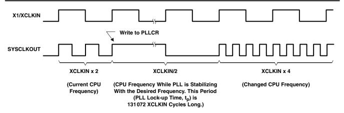
Figure 6-11. Effect of Writing Into PLLCR Register
