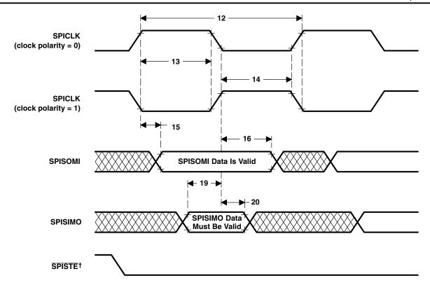
$<sup>^{\</sup>dagger}$  In the slave mode, the  $\overline{\text{SPISTE}}$  signal should be asserted low at least 0.5t\_{c(SPC)} before the valid SPI clock edge and remain low for at least 0.5t\_{c(SPC)} after the receiving edge (SPICLK) of the last data bit.
