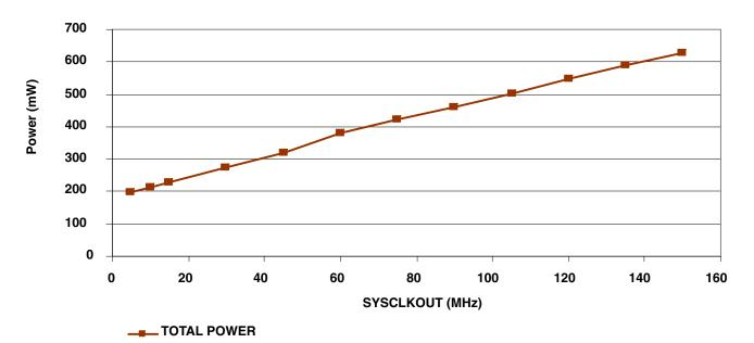
Figure 6-1. Typical Current Consumption Over Frequency
