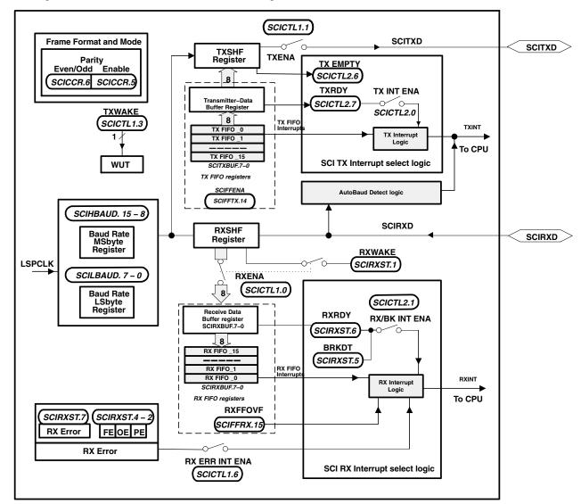
Figure 4–10 shows the SCI module block diagram.
