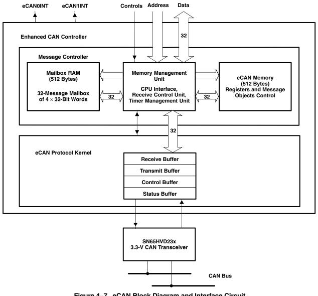
Figure 4–7. eCAN Block Diagram and Interface Circuit
