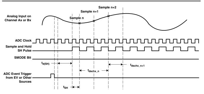
Figure 6–38. Sequential Sampling Mode (Single-Channel) Timing
