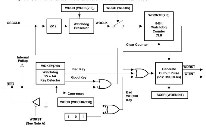
NOTE A: The  $\overline{\text{WDRST}}$  signal is driven low for 512 OSCCLK cycles.
