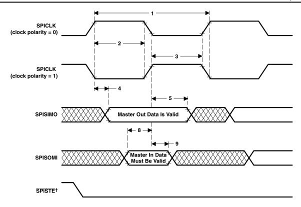
$<sup>^{\</sup>dagger}$  In the master mode,  $\overline{\text{SPISTE}}$  goes active  $0.5t_{\text{c(SPC)}}$  before valid SPI clock edge. On the trailing end of the word, the  $\overline{\text{SPISTE}}$  will go inactive  $0.5t_{\text{c(SPC)}}$  after the receiving edge (SPICLK) of the last data bit.
