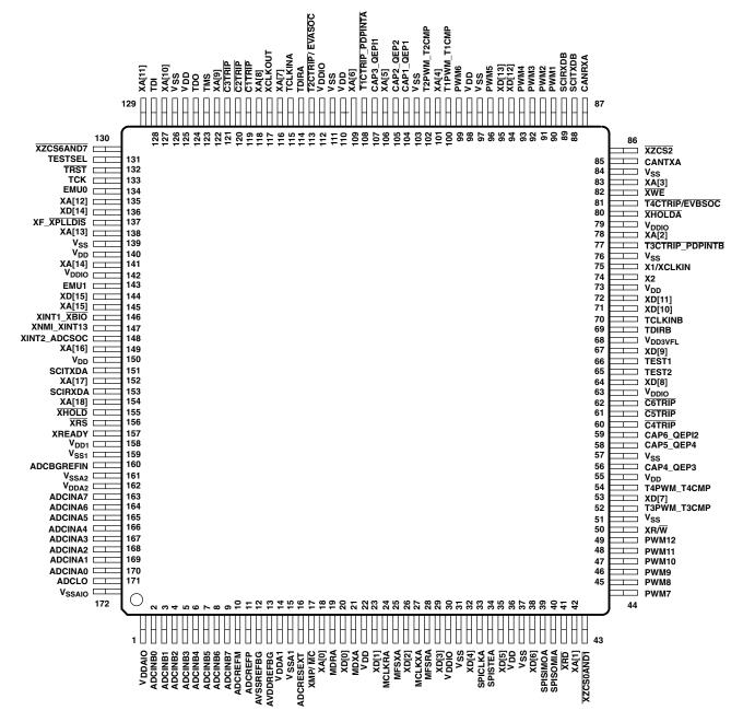
Figure 2-1. SM320F2812 172-Pin HFG CQFP (Top View)
