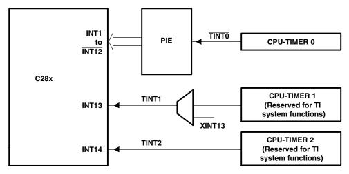
NOTES: A. The timer registers are connected to the Memory Bus of the C28x processor.
