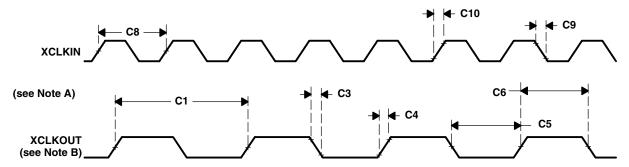
NOTES: A. The relationship of XCLKIN to XCLKOUT depends on the divide factor chosen. The waveform relationship shown in Figure 6–7 is intended to illustrate the timing parameters only and may differ based on configuration.
