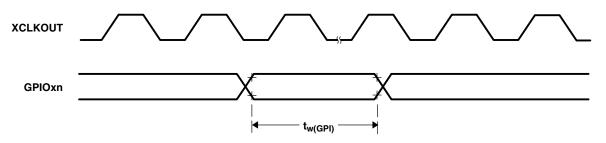
Figure 6-22. General-Purpose Input Timing
