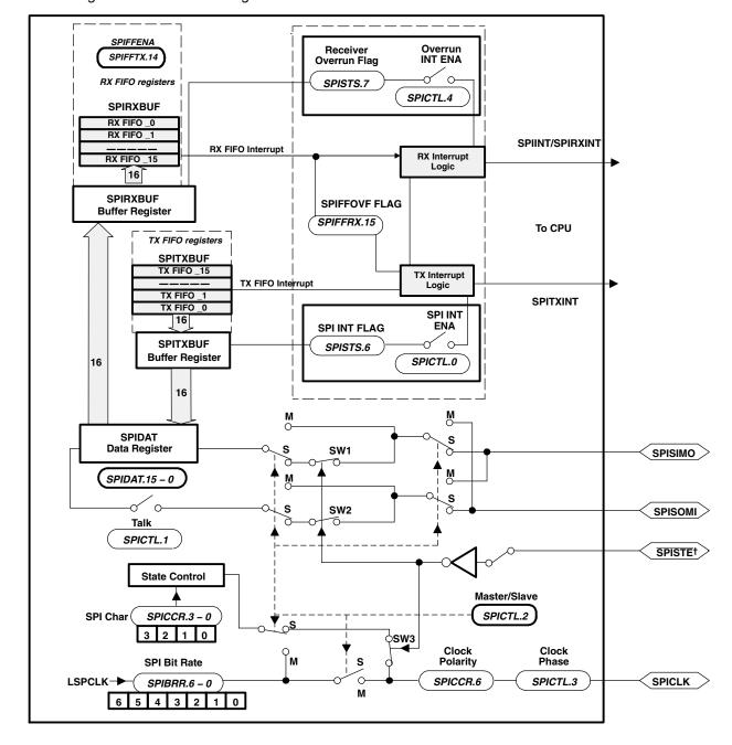
Figure 4–11 is a block diagram of the SPI in slave mode.
