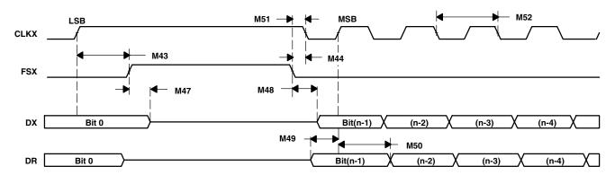
Figure 6-44. McBSP Timing as SPI Master or Slave: CLKSTP = 10b, CLKXP = 1
