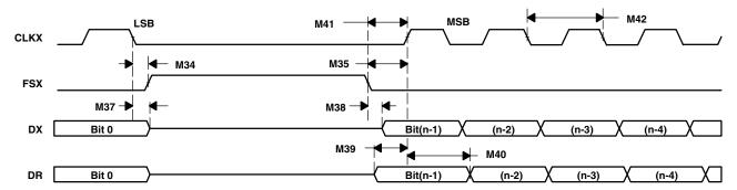
Figure 6-43. McBSP Timing as SPI Master or Slave: CLKSTP = 11b, CLKXP = 0
