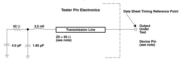
NOTE: The data sheet provides timing at the device pin. For output timing analysis, the tester pin electronics and its transmission line effects must be taken into account. A transmission line with a delay of 2 ns or longer can be used to produce the desired transmission line effect. The transmission line is intended as a load only. It is not necessary to add or subtract the transmission line delay (2 ns or longer) from the data sheet timing.
