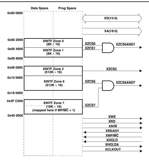
NOTES: A. The mapping of XINTF Zone 7 is dependent on the XMP/MC device input signal and the MP/MC mode bit (bit 8 of XINTCNF2 register). Zones 0, 1, 2, and 6 are always enabled.
