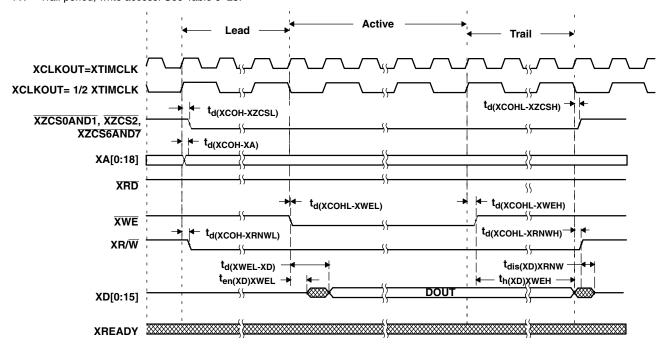
NOTES: A. All XINTF accesses (lead period) begin on the rising edge of XCLKOUT. When necessary, the device inserts an alignment cycle before an access to meet this requirement.
