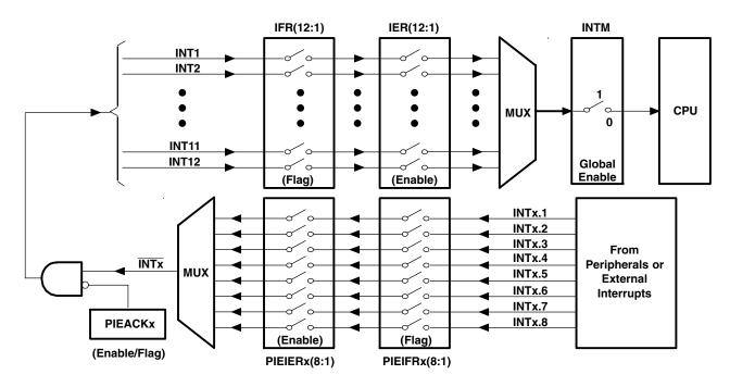
Figure 3–5. Multiplexing of Interrupts Using the PIE Block
