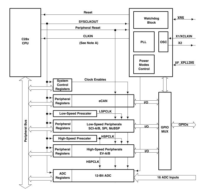
NOTE A: CLKIN is the clock input to the CPU. SYSCLKOUT is the output clock of the CPU. They are of the same frequency.
