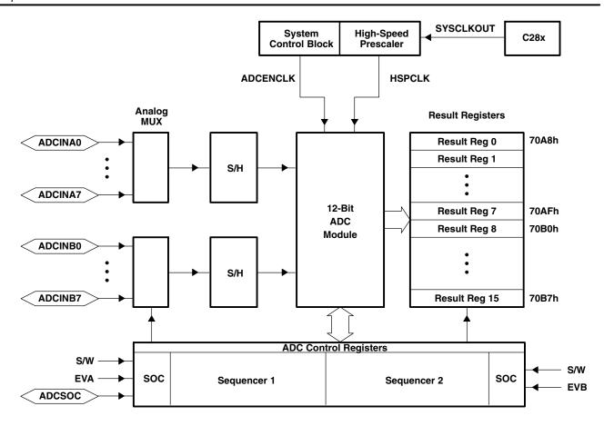
Figure 4-4. Block Diagram of the F2812 ADC Module
