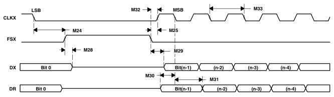
Figure 6-42. McBSP Timing as SPI Master or Slave: CLKSTP = 10b, CLKXP = 0
