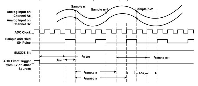
Figure 6-39. Simultaneous Sampling Mode Timing
