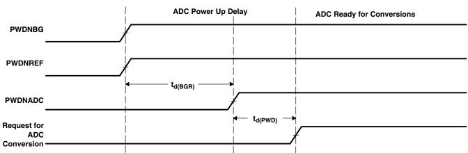
Figure 6-37. ADC Power-Up Control Bit Timing
