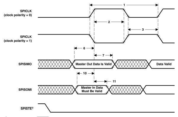
$<sup>^{\</sup>dagger}$  In the master mode,  $\overline{\text{SPISTE}}$  goes active  $0.5t_{\text{c(SPC)}}$  before valid SPI clock edge. On the trailing end of the word, the SPISTE goes inactive  $0.5t_{\text{c(SPC)}}$  after the receiving edge (SPICLK) of the last data bit.
