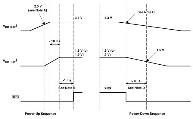
$<sup>\</sup>begin{array}{llll} \dagger \ V_{DD\_3.3V} & - & V_{DDIO}, \ V_{DD3VFL}, \ V_{DDAIO}, \ V_{DDA1}, \ V_{DDA2}, \ AV_{DDREFBG} \\ \dagger \ V_{DD\_1.8V} & - & V_{DD}, \ V_{DD1} \end{array}$
