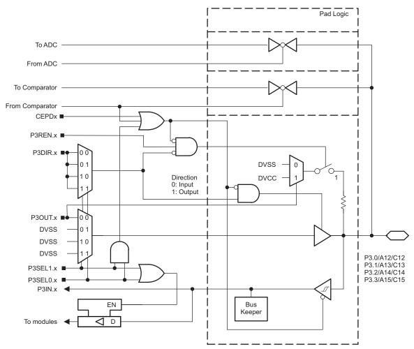
Figure 5-9. Port P3 (P3.0 to P3.3) Diagram
