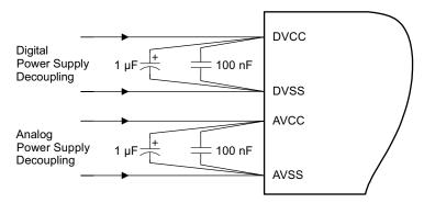
Figure 6-1. Power Supply Decoupling
