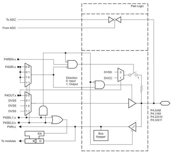
Figure 5-11. Port P4 (P4.0 to P4.3) Diagram
