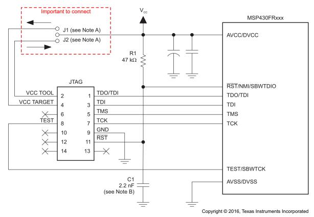
If a local target power supply is used, make connection J1. If power from the debug or programming adapter is used, make connection J2.
