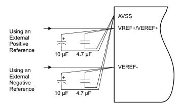
Figure 6-5. ADC12\_B Grounding and Noise Considerations
