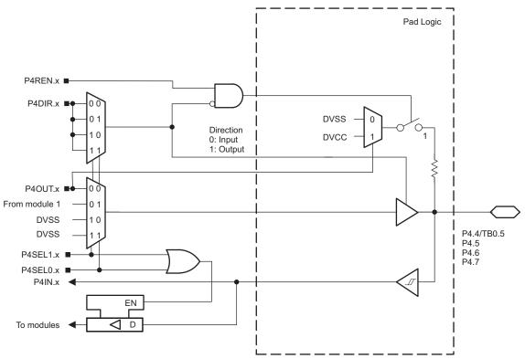
Figure 5-12. Port P4 (P4.4 to P4.7) Diagram
