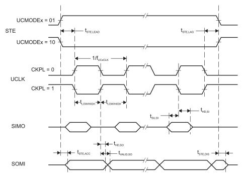
Figure 4-14. SPI Slave Mode, CKPH = 1
