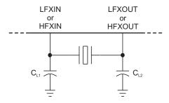
Figure 6-2. Typical Crystal Connection
