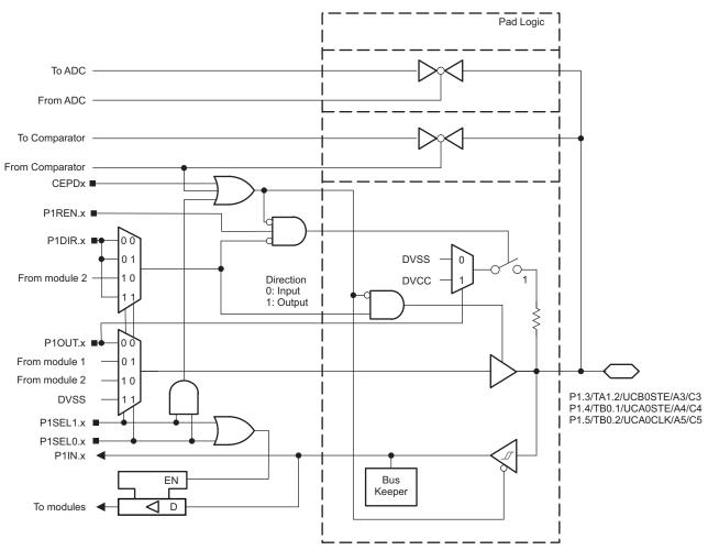
Figure 5-3. Port P1 (P1.3 to P1.5) Diagram
