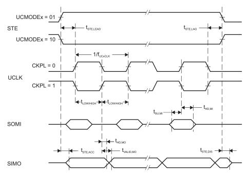
Figure 4-12. SPI Master Mode, CKPH = 1
