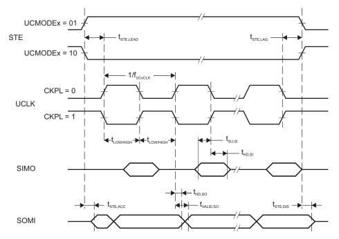
Figure 4-13. SPI Slave Mode, CKPH = 0
