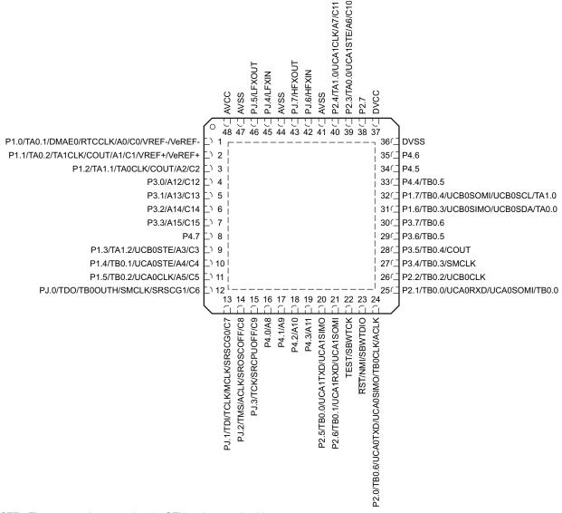
NOTE: TI recommends connecting the QFN package pad to V<sub>SS</sub>. NOTE: On devices with UART BSL: P2.0: BSLTX; P2.1: BSLRX. NOTE: On devices with I<sup>2</sup>C BSL: P1.6: BSLSDA; P1.7: BSLSCL.
