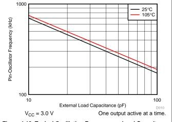
Figure 4-9. Typical Oscillation Frequency vs Load Capacitance
