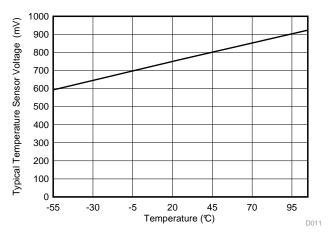
Figure 4-16. Typical Temperature Sensor Voltage
