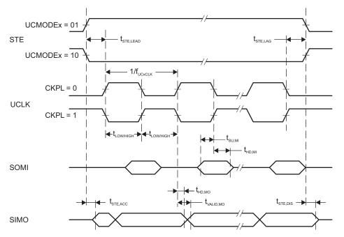
Figure 4-11. SPI Master Mode, CKPH = 0
