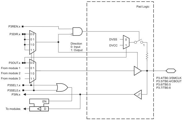
Figure 5-10. Port P3 (P3.4 to P3.7) Diagram
