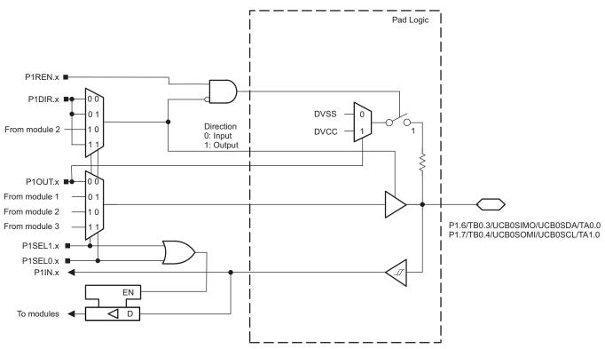
Figure 5-4. Port P1 (P1.6 and P1.7) Diagram
