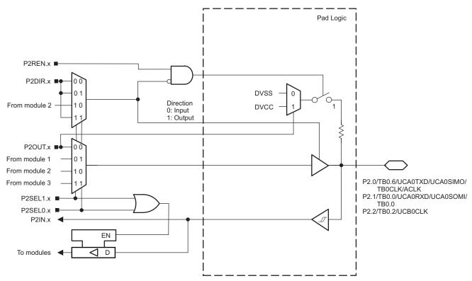
Figure 5-5. Port P2 (P2.0 to P2.2) Diagram
