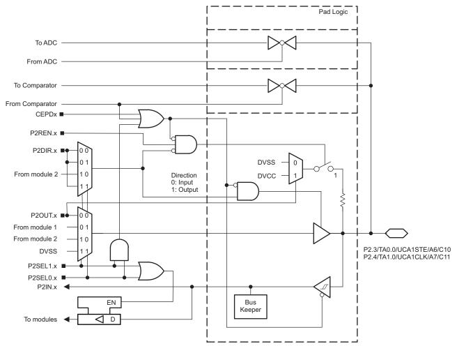
Figure 5-6. Port P2 (P2.3 and P2.4) Diagram
