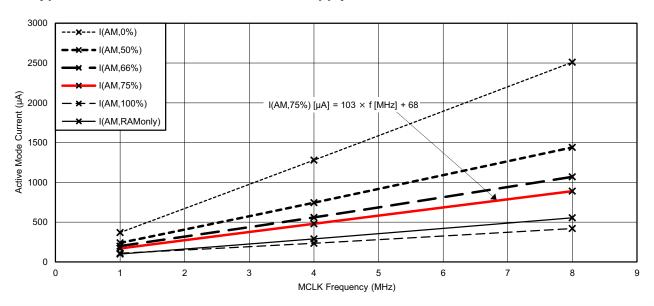
NOTE: I(AM, cache hit ratio): Program resides in FRAM. Data resides in SRAM. Average current dissipation varies with cache hit-to-miss ratio as specified. Cache hit ratio represents number cache accesses divided by the total number of FRAM accesses. For example, a 75% ratio implies three of every four accesses is from cache, and the remaining are FRAM accesses.
