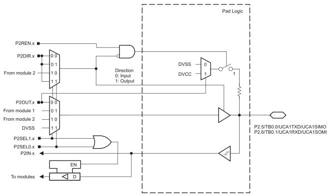
Figure 5-7. Port P2 (P2.5 and P2.6) Diagram
