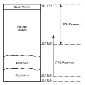
Figure 5-1. Interrupt Vectors, Signatures and Passwords
