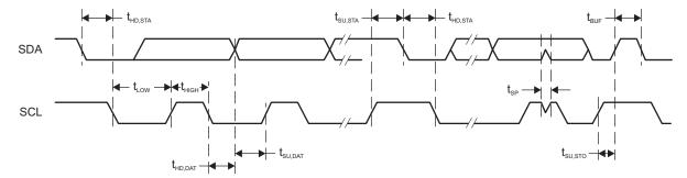
Figure 4-15. I<sup>2</sup>C Mode Timing
