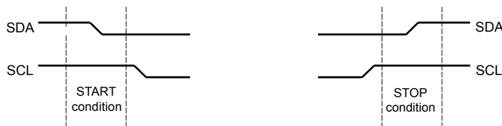
Figure 14-3. START and STOP Conditions
