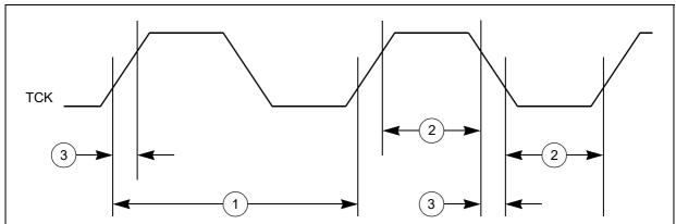
Figure 13. JTAG test access port timing
