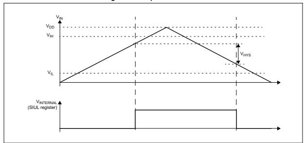
Figure 3. I/O input electrical characteristics
