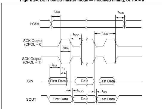
Figure 24. DSPI CMOS master mode — modified timing, CPHA = 0
