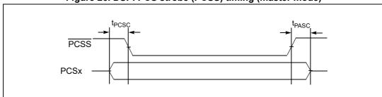
Figure 26. DSPI PCS strobe (PCSS) timing (master mode)
