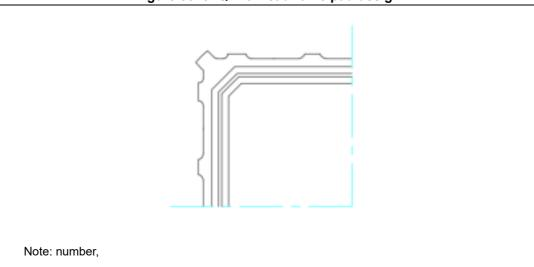
Figure 33. eTQFP64 leadframe pad design
