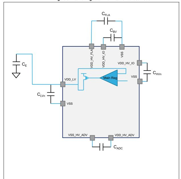
Figure 9. Internal regulator with internal ballast mode
