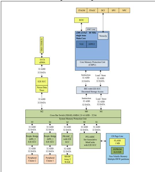
Figure 1. Block diagram
