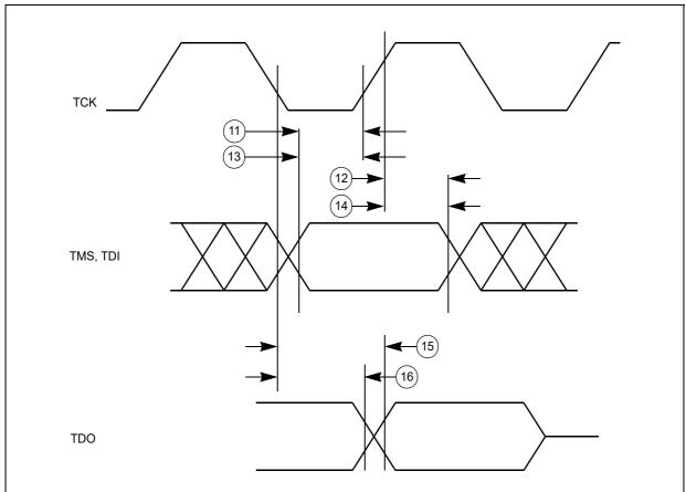
Figure 18. Nexus TDI, TMS, TDO timing
