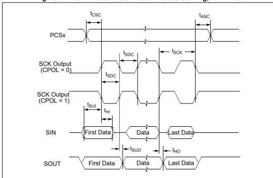
Figure 21. DSPI CMOS master mode — classic timing, CPHA = 0
