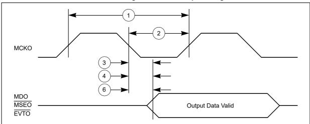
Figure 17. Nexus event trigger and test clock timings
