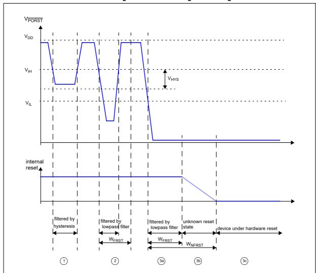
Figure 6. Noise filtering on reset signal
