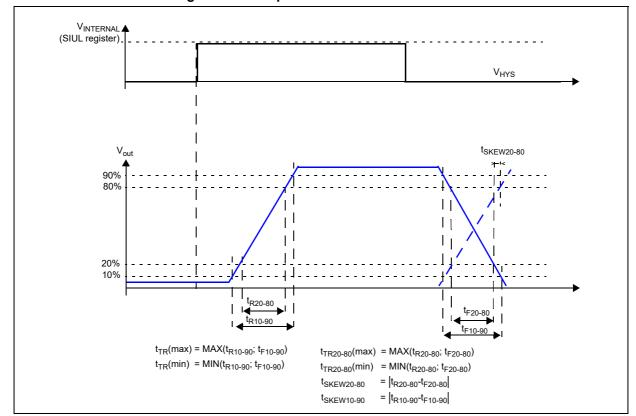
Figure 4. I/O output DC electrical characteristics definition
