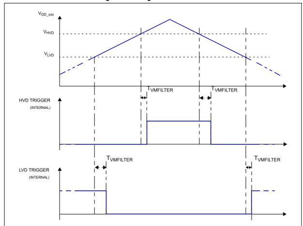
Figure 11. Voltage monitor threshold definition
