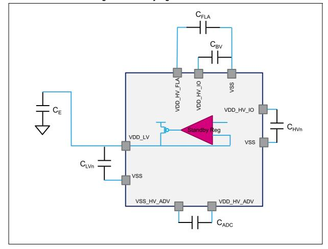
Figure 10. Standby regulator with internal ballast mode
