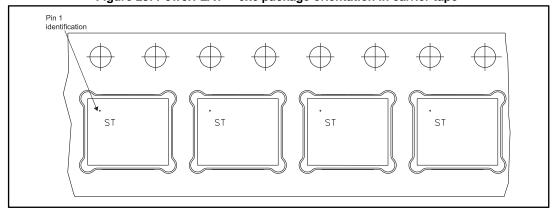
Figure 24: PowerFLAT™ 5x6 reel
