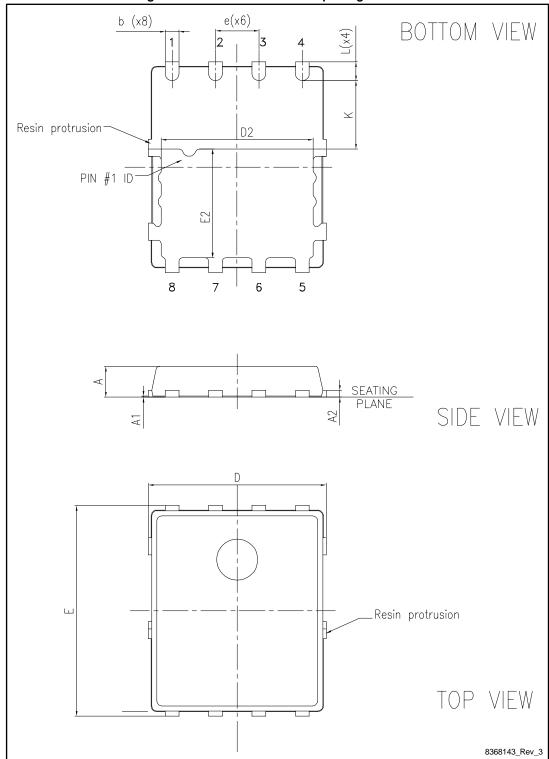
Table 9: PowerFLAT™ 5x6 HV mechanical data
