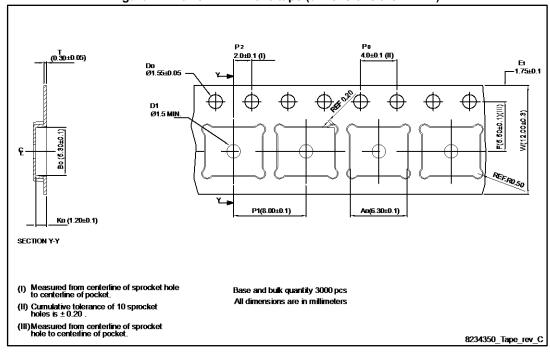
Figure 23: PowerFLAT™ 5x6 package orientation in carrier tape
