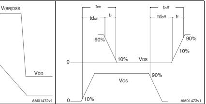
Figure 18. Switching time waveform
