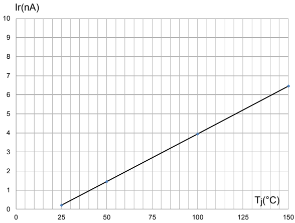
Figure 2. Leakage current versus junction temperature at V_{RM} 20 V (typical value)
