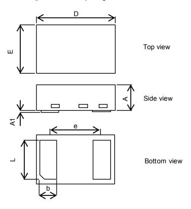
Table 3. SOD882T package mechanical data
