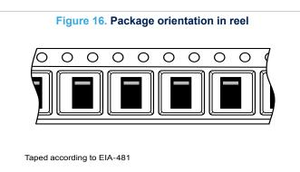
Note: Pocket dimensions are not on scale Pocket shape may vary depending on package On bidirectional devices, marking and logo may be not always in the same direction
